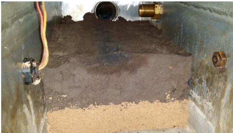
*Figure 2-1 Decontamination cross section for a 10 MeV beam into a high-clay-content 5% contaminated soil [2-28].*
