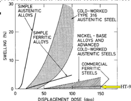
Figure 29: Swelling comparisons between HT-9 and other potential cladding materials.
