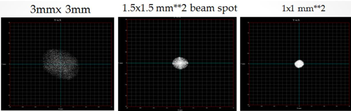
Figure 7: TRACE 3D simulations for the beam from the source to the LEBT. The accelerator group optimized the solenoid settings of Trace-3D such that the output of the simulation provides the design value given by LANL scientists during design and commissioning of the LEDA.
