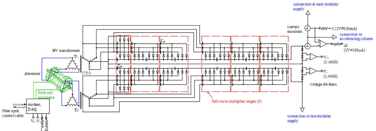
FIGURE 2. Circuit of one CMA module.
