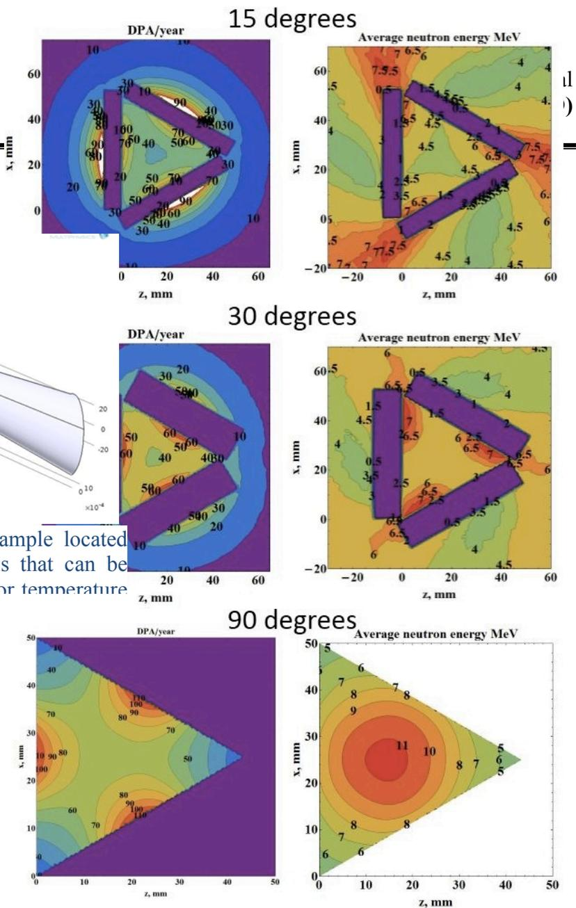
Figure 21: The three beam of the SFC are aimed at different angles producing different mean energies for the sample area that can hold 21 samples. The angle indicated is off the target fave and are all arranged clockwise. The mean energy are as follows: 15 deg – 4.5 MeV, 30 deg – 5.5 meV, and 90 deg – 8
