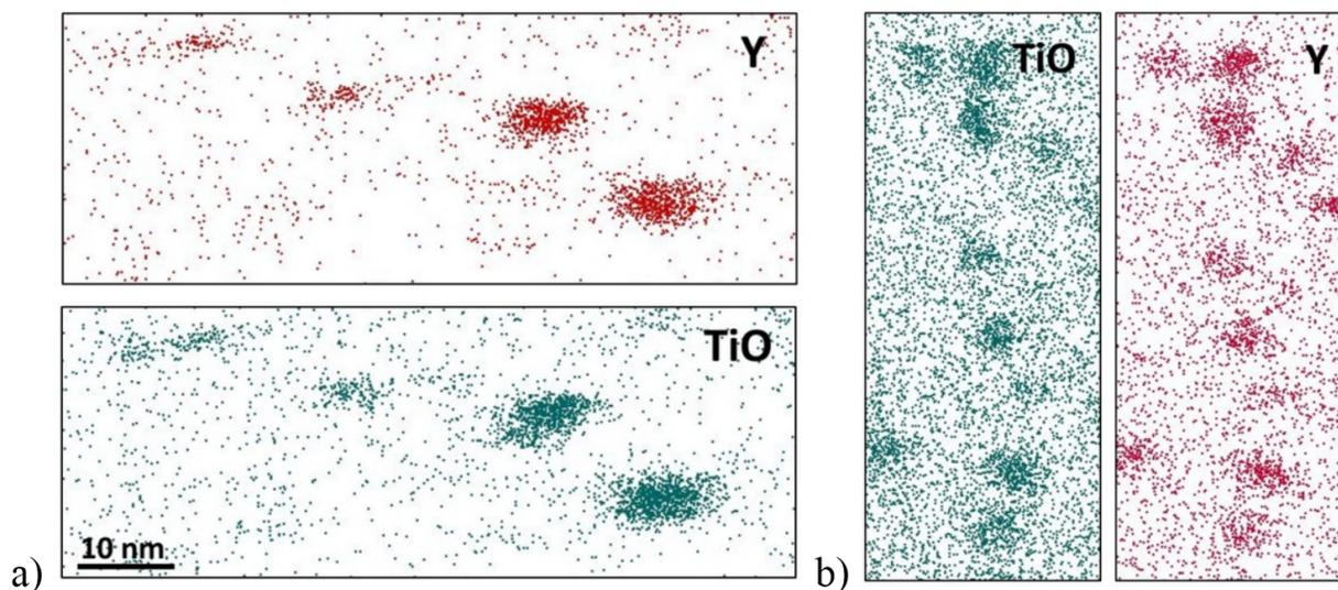
Figure 35: Atomic probe tomography (APT) elemental maps of the (a) as-received (un-irradiated) 9%Cr ODS and (b) neutron irradiated 9%Cr ODS to 3 dpa at 500°C showing
