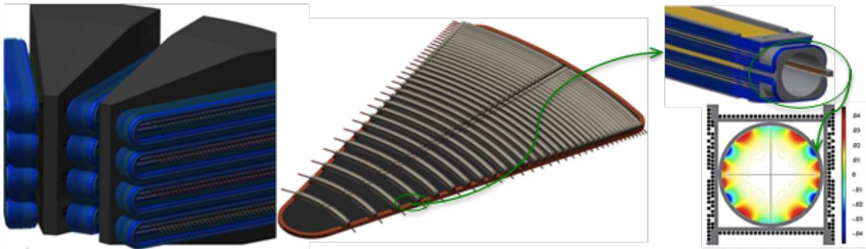
Figure 13: Left Superconducting cavities in blue. Middle: a sector magnet with a FODO lattice of quad focusing channels which tightly control the beam to allow high current. Right: close up of Quad and magnetic field cross section.
