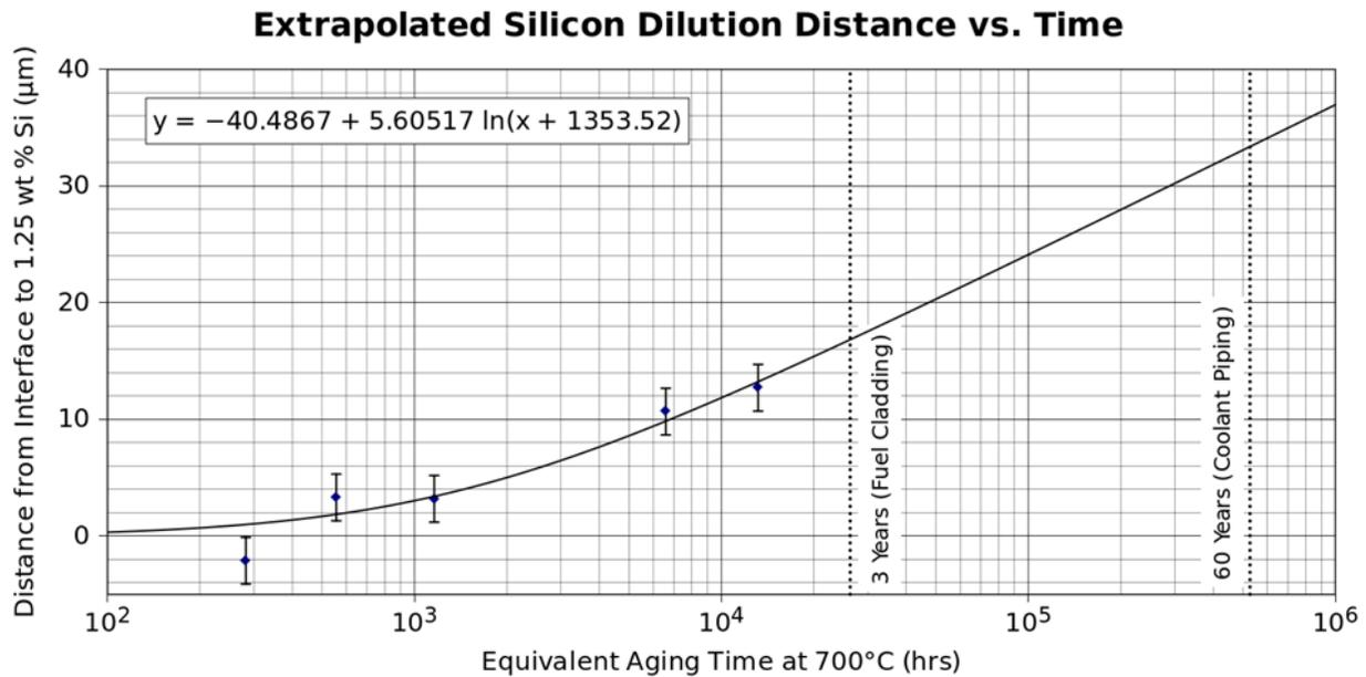
Figure 27: Extrapolated distance of minimum Si content to maintain FGC corrosion resistance at 700 C vs. time (39)
