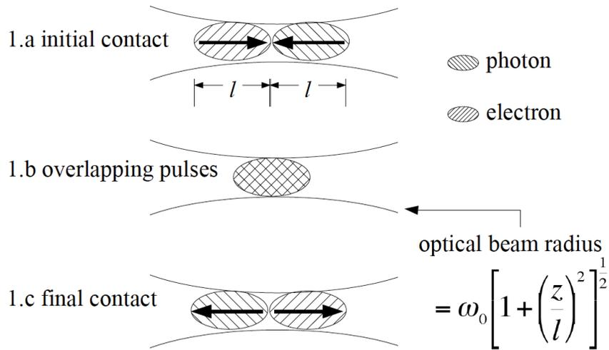
Figure 1. Electrons moving through an optical pulse with a depth of field (Rayleigh parameter) equal to the pulse length  $l$  see a nearly constant beam radius.
