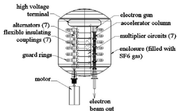
FIGURE 1. Cross section of CMA system.
