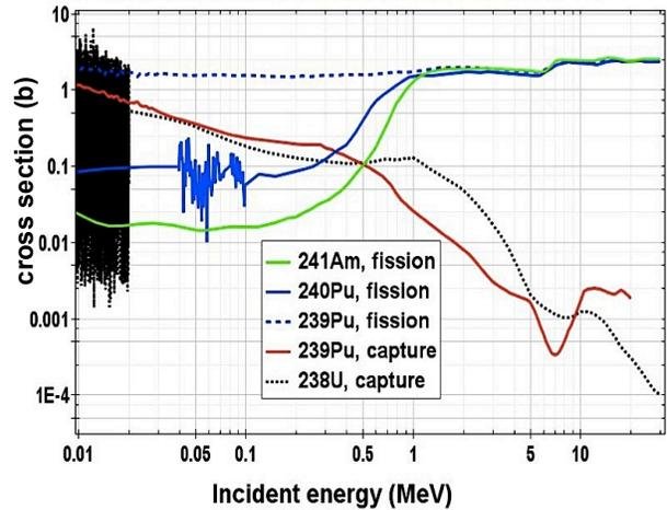
Figure 3. Energy dependence of cross sections for fission and capture by  $^{238}\text{U}$  and the dominant transuranics.
