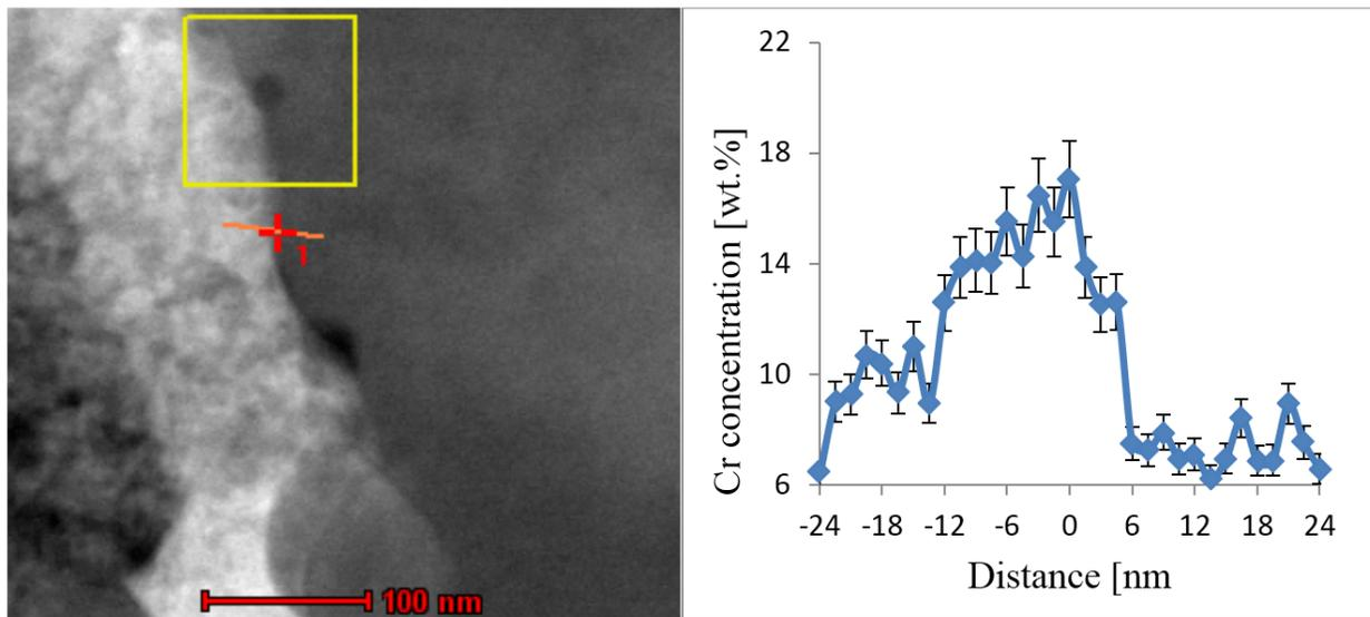
Figure 34: STEM image of a PAGB of NF616 steel neutron irradiated at 3 dpa at 500oC (left) and corresponding line scan for chromium composition across PAGB (right).
