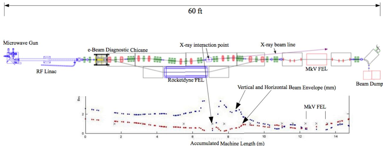
Figure 3. Scale drawing to University of Hawai'i optimized inverse-Compton x-ray source: beam line schematic and the micro focus solution.
