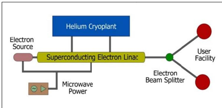
Figure 2. Conceptual Layout of the Niowave Superconducting Electron Linac used for various applications
