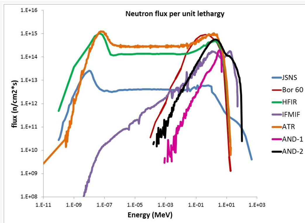
Figure 15: Comparison of the neutron flux and energy spectrum of various facilities around the world, and those currently under design.
