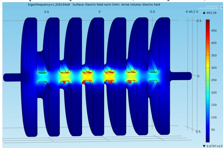
Figure 12: First iteration of the 6 cell kicker for the separation strategy. This cavity can provide 2 degrees of deflec-
