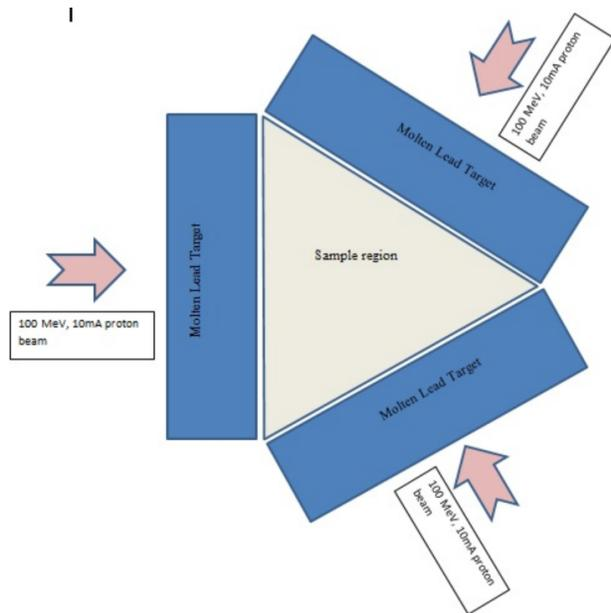
Figure 18: Diagram of the AND-2 irradiation chamber.
