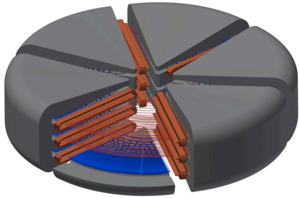
Figure 5. 3-stack of 100 MeV strong-focusing cyclotrons, with cutaway to show cavities, BTCs, and orbits.
