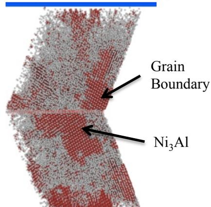
Figure 37: Monte Carlo simulation of Ni<sub>3</sub>Al precipitation, next to a grain boundary in a Ni-0.10at.Al at 900K.
