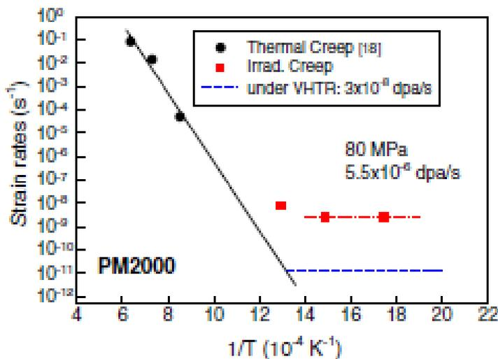
Figure 20: Temperature dependence of creep rates of PM2000 without irradiation (solid line), under He-implantation (dash-dotted), and expected for VHTR conditions (dashed line).[3]
