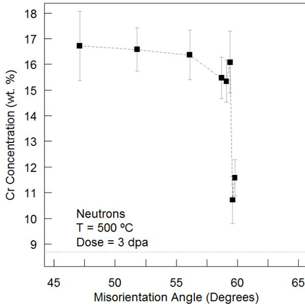
Figure 33: On-boundary Cr concentration in Fe-9%Cr binary alloy as a function of misorientation for high angle grain boundaries near the  $\Sigma 2$  axis
