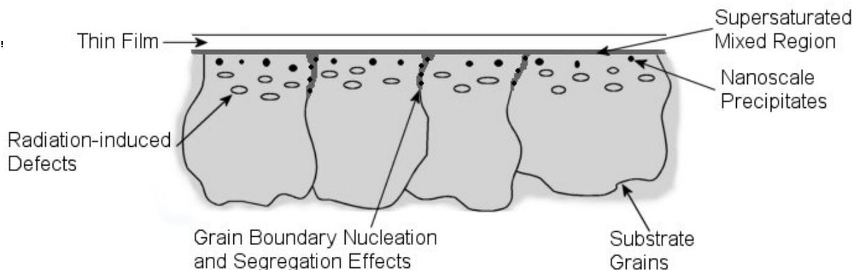
Figure 30: Types of irradiation damage at near interface area
