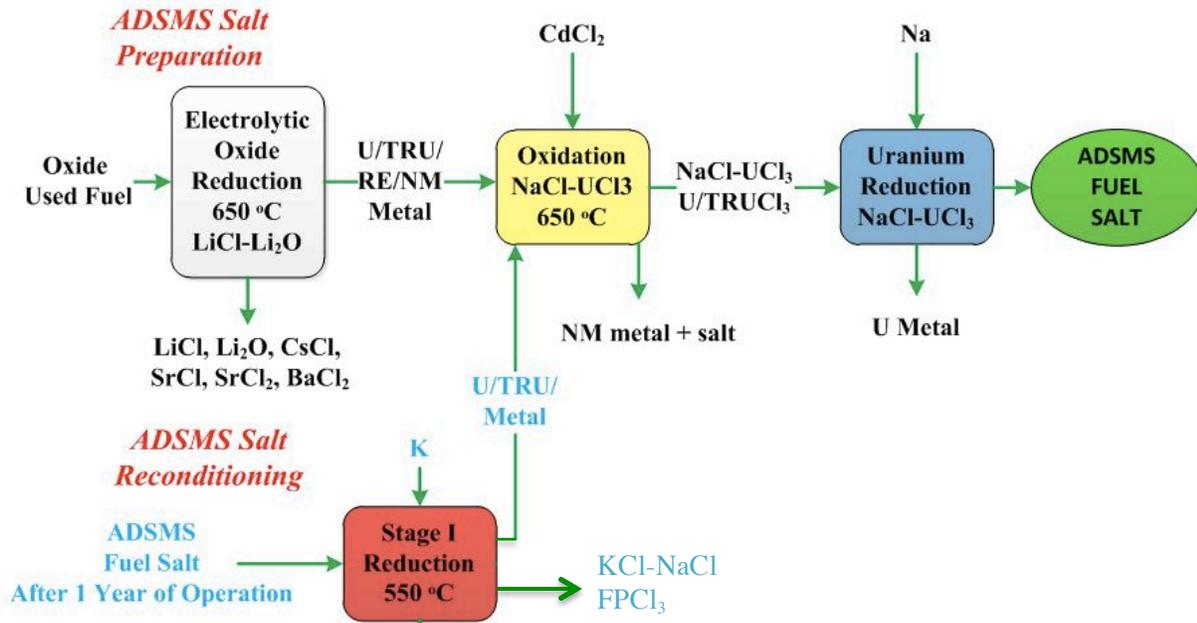
Figure 2. Pyroprocessing and electro-separation processes used to prepare the fuel salt.
