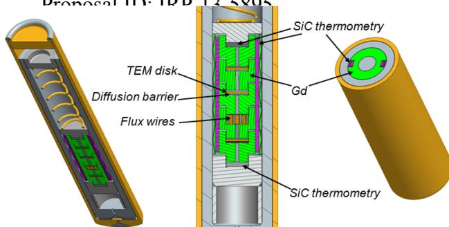
Figure 16: HFIR Irradiation Capsule Design for a Previous Texas A&M University Fast Neutron Irradiation
