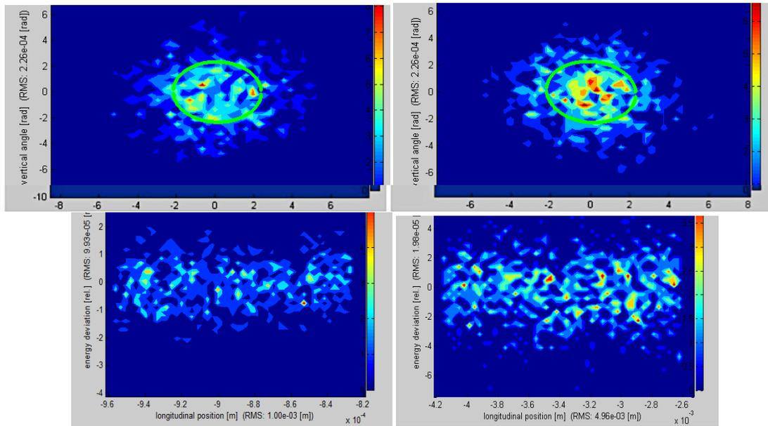
Figure 6. a) Beam breakup in transverse phase space after 2<sup>nd</sup> orbit when tune is near 3<sup>rd</sup> order and 5<sup>th</sup>-order resonances; b) beam breakup in longitudinal phase space when tune is near 5<sup>th</sup> order resonance.
