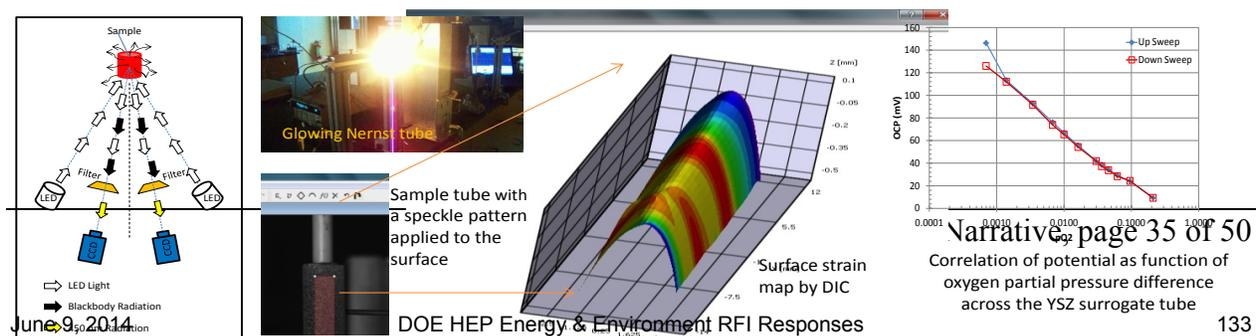
Figure 32: Preliminary study on the internal pressure test using a solid Nernst glower tube.
