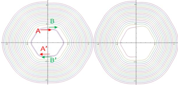
Figure 3. Reference orbits in the 6-sector TAMU100, before and after optimization of the injection orbit.
