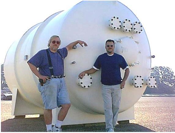
**FIGURE 4.** Pressure tank for 1 MV, 100 kW CMA.
