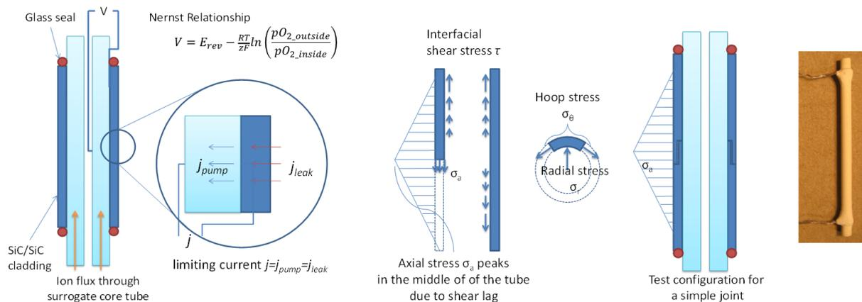
Figure 31: Proposed test schemes for SiC/SiC cladding tube and joint using a surrogate core tube; (right) a Nernst glower bar: L=45mm, dia=2.7 mm in dia.
