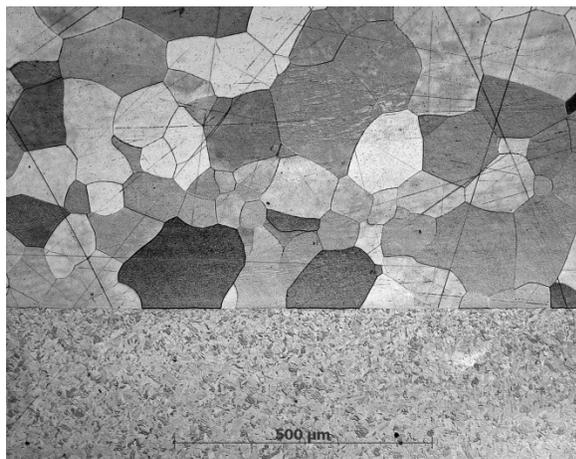
Figure 28: Micrograph of the as manufactured FGC, 100x. Irradiation induced mixing is a key concern for the FGC (39).
