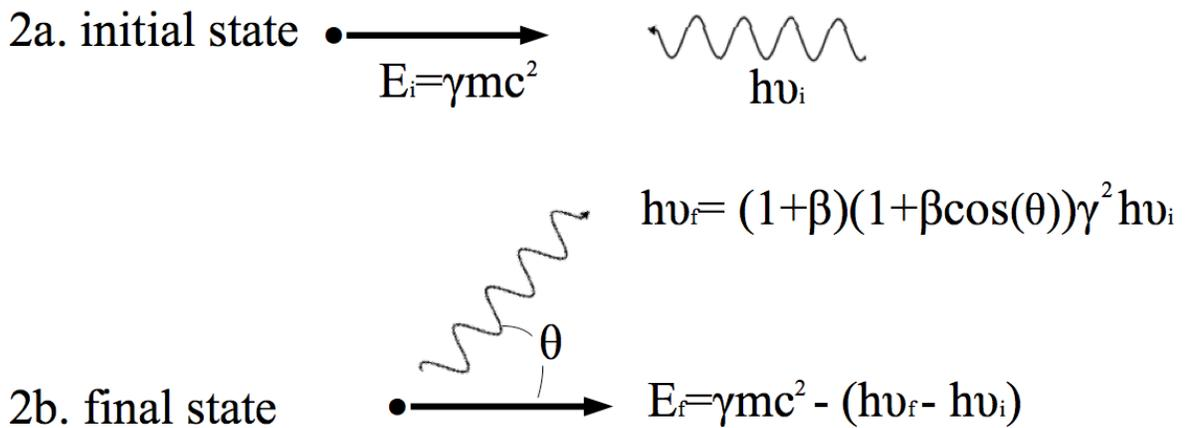
Figure 2. Relationship of the scattering angle  $\theta$ , initial and final photon and electron energies.
