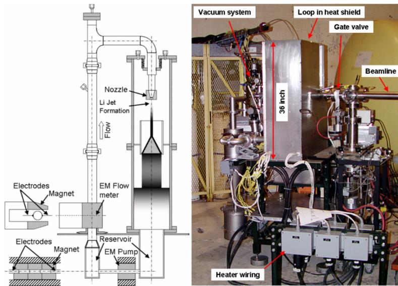
Figure 14: Schematic and picture of the Lithium target constructed at Argonne National lab (2).
