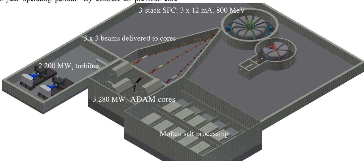
Figure 8. 3-core ADAM facility that destroys transuranics at the same rate they are produced by a  $\text{GW}_e$  nuclear power
