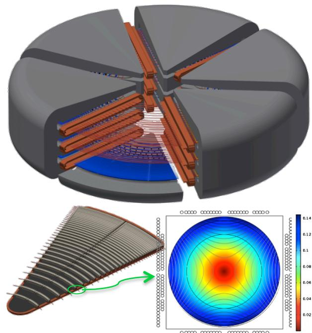
Figure 1. a) 3-stack of 100 MeV SFCs, with cutaway to show superconducting cavities, BTCs, and orbits; b) detail of a sector dipole flux plate and the arced BTCs.
