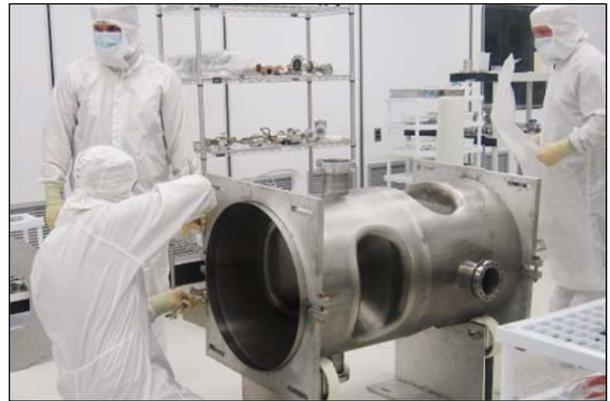
Figure 1. A niobium superconducting accelerating structure being processed in the Niowave cleanroom
