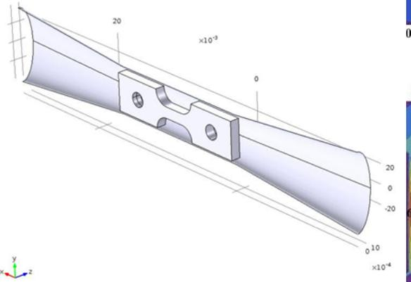
Figure 22: Miniature tensile sample located within a cooling/fluid channels that can be inserted into the neutron flux for temperature design
