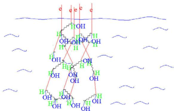
**FIGURE 7.** Ionization cascade in water makes free radicals.
