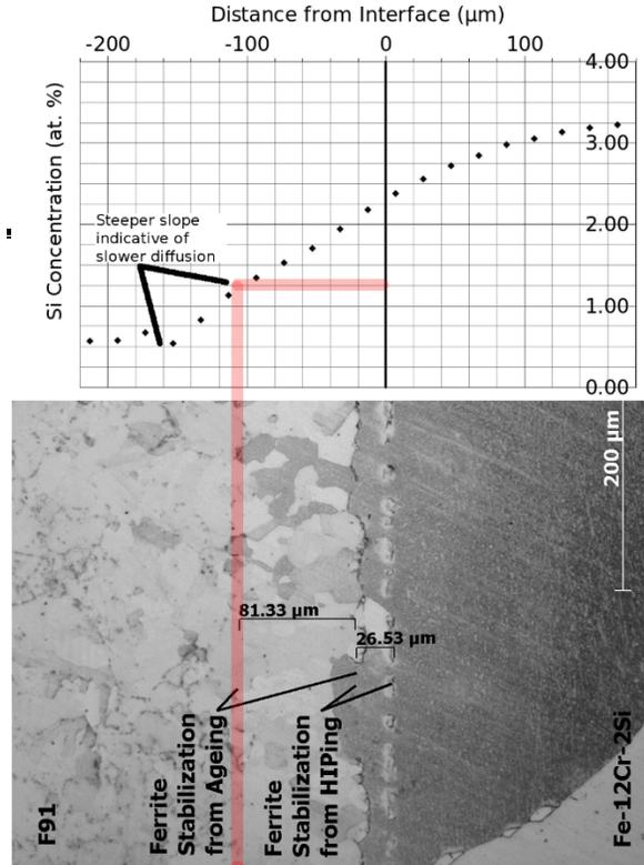
Figure 26: FGC diffusion couple aged at 800°C for 600hr, with Si concentration profile. The graph shows a steeper slope indicative of slower diffusion near the interface. The micrograph shows the interface between F91 and Fe-12Cr-2Si, with regions of ferrite stabilization from ageing and HIPing. A red vertical line marks the interface. Distances of 81.33 μm and 26.53 μm are indicated from the interface to specific points in the F91 region. A 200 μm scale bar is shown on the right.
