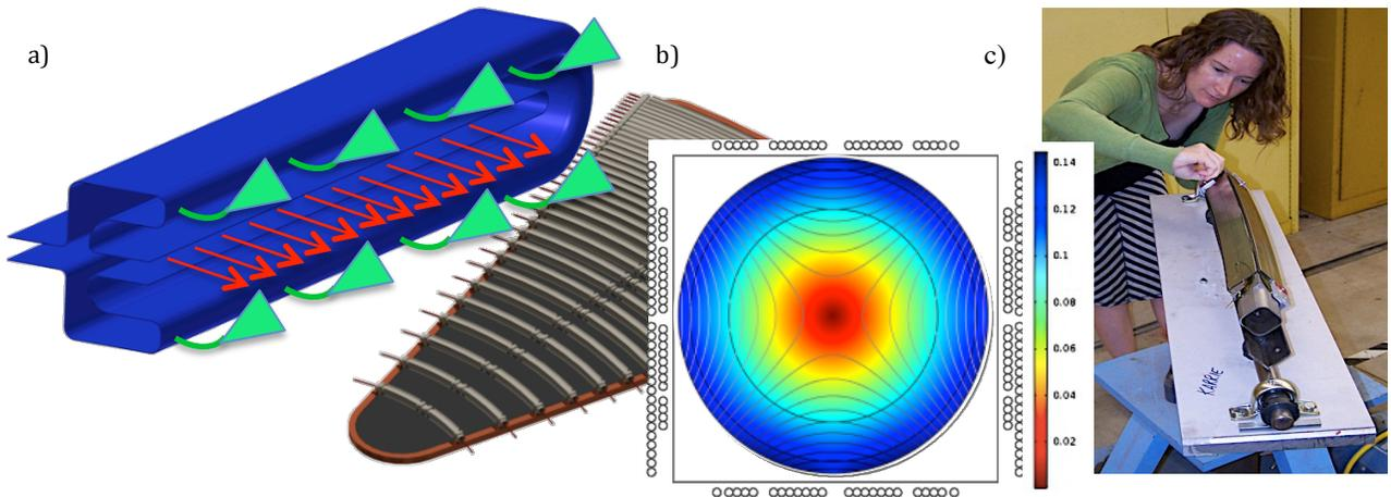
Figure 6. Innovations in the strong-focusing cyclotron: a) 117 MHz  $\frac{1}{4}$ -wave superconducting cavity with linear array of input couplers (green); b) beam transport channels on a flux plate; c) detail of the  $\text{MgB}_2$  windings on a BTC and its quadrupole field distribution (max gradient 6 T/m).
