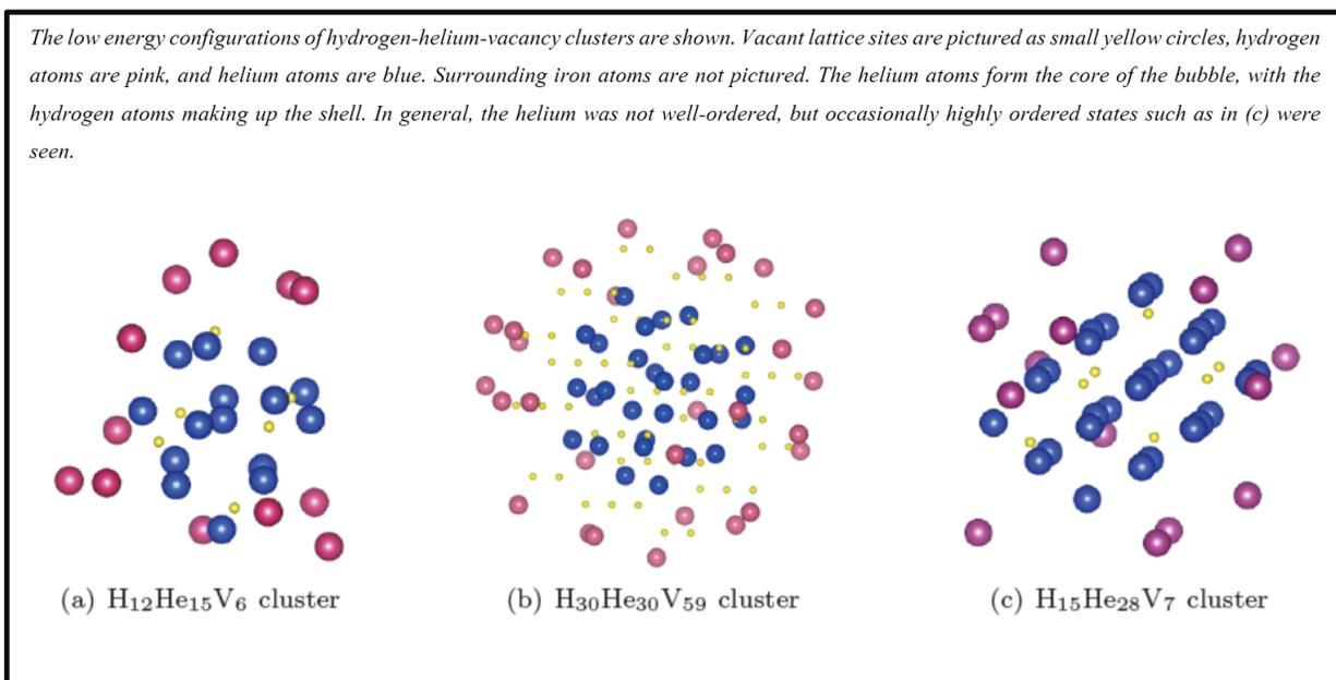
Figure 36: Examples of model dynamics of H, He, vacancy clusters during neutron damage.
