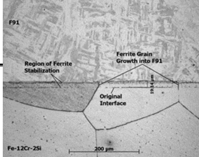
Figure 25: As-HIPed diffusion couple of the FGC, 100x (39)
