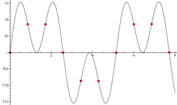
Figure 11: The spectrometer system uses two cavities operating at 58.3 MHz and another at 175 MHz to either increase or decrease the energy to allow different trajectories for 3 beams in the uniform magnetic field. The graph is an overlay of the two modes with the bunches indicated in red. The three beams (+,-,0) all have two bunches each. A single cavity (58.3 MHz) could be used if the particle speed were higher
