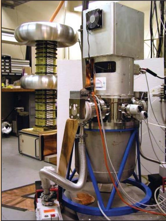
Figure 19. A 165-keV electrostatic accelerator with high-voltage power supply (in background on left). Figure courtesy of Arlyn Antolak, Sandia National Laboratories.
