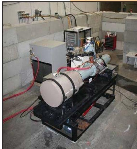
Figure 18. A transportable, forward dose-controlled, photon inspection system prototype using a nominal 30-MeV LINAC mounted on a  $2.4 \times 1.2$ -m beam targeting assembly for standoff nuclear material detection. Figure courtesy of James L. Jones, Idaho National Laboratory.
