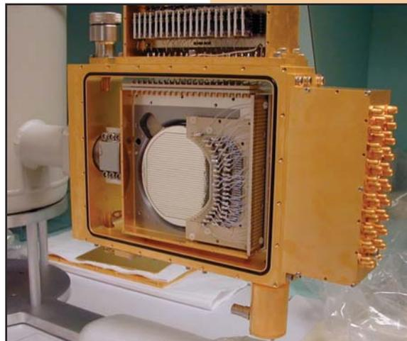
Figure 15. Photograph of a germanium double-sided strip detector [Vet06]. This particular detector has 38 strips on each side and thus contains 1,444 effective pixels, yet is read out into only 76 channels. This particular detector has an active area of about 50 cm<sup>2</sup> and is 11-mm thick. Figure courtesy of Kai Vetter, Lawrence Berkeley National Laboratory.
