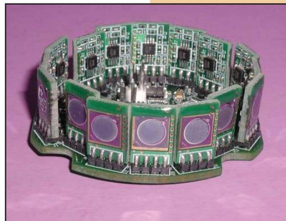
Figure 6. Photograph of an array of silicon-based conversion layer detectors, the 6-mm-diameter circles attached to each circuit board. Figure courtesy of Douglas McGregor, Kansas State University.
