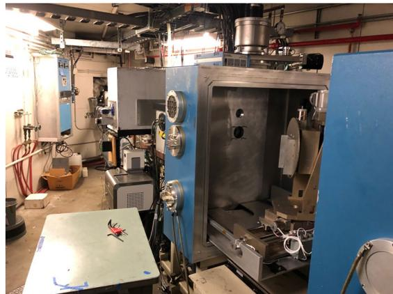
Figure 48: Example of an existing facility for heavy ion irradiation. Beam enters from the back of the frame. Large blue vacuum chamber holds device under test. Vacuum feedthroughs are at the left of the chamber. Remote movable stages are seen on a sliding platform. Such capabilities and facilities, specifically targeting the conditions of future colliders are required going forward.
