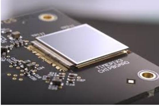
Figure 43: Example of a hybrid pixel detector: the silicon sensor is connected to the readout electronics fabricated on a silicon wafer via “bump-bonds” that connect the sensor electrodes to the inputs of the sensor. This structure allows for comparable resolution in two dimensions. Here the TIMEPIX3 cell is shown [273], it features a square pixel size of  $55 \times 55 \mu\text{m}$ .
