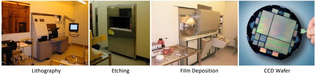
Figure 55: Photographs of the various processing bays of the Micro-Systems laboratory at LBNL with a picture of a fully processed CCD wafer. (photo credit: LBNL).
