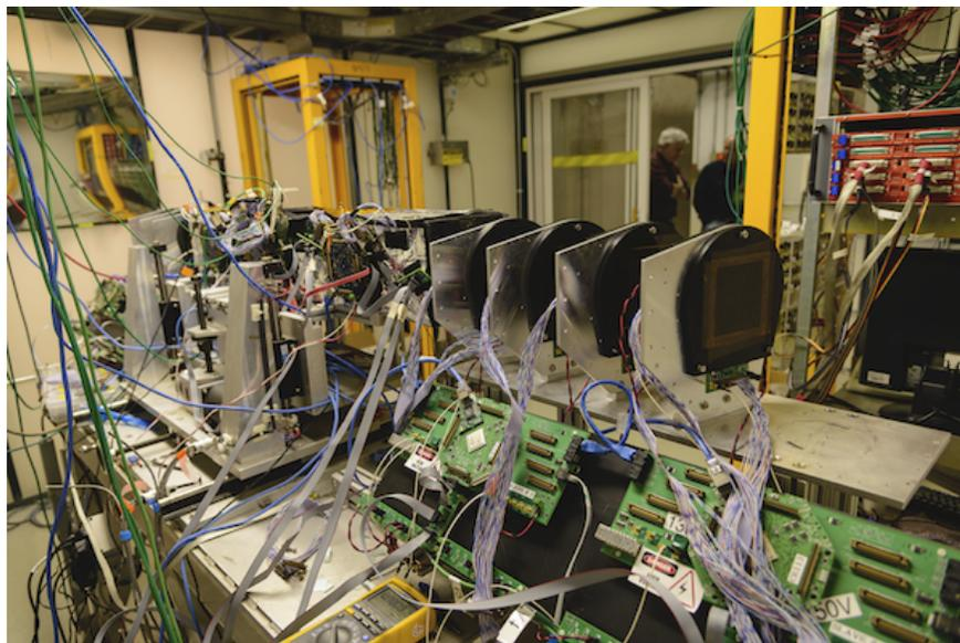
Figure 54: Experimental setup in the Fermilab Test Beam Facility (photo credit: Fermilab).
