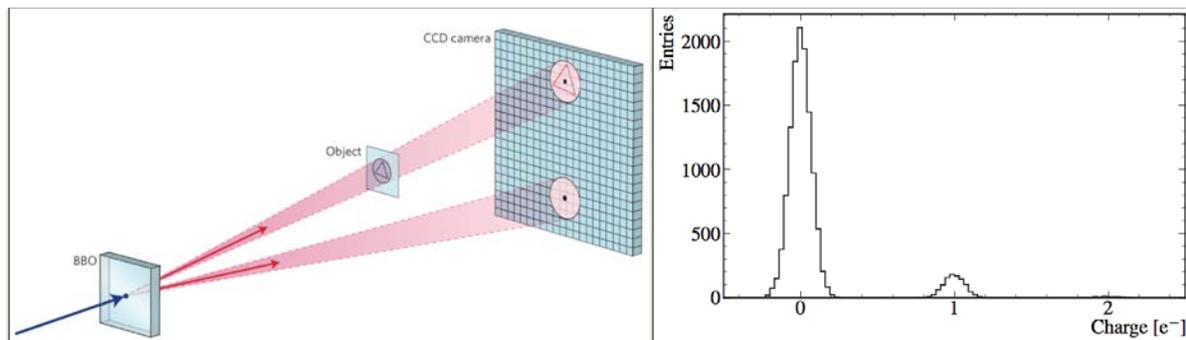
**Figure 1.** Left) The differential quantum imaging experiment. The  $\beta$ -barium borate (BBO) crystal produced an entangled pair which is then imaged with a CCD camera. Non-classical correlations are used for the improved differential imaging of a weakly absorbing object. [Figure from Nature Photonics] Right) Photon counting capabilities of the skipper-CCD, showing the signal for zero and 1 photo-electrons.
