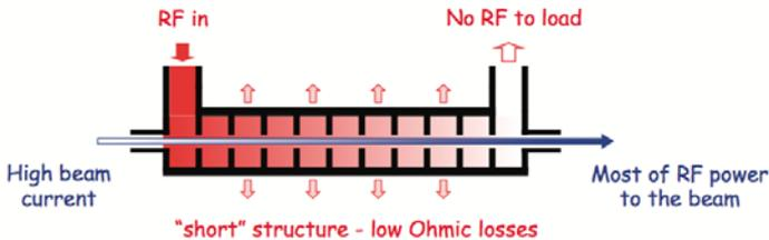
High current, full-loaded linac operation
