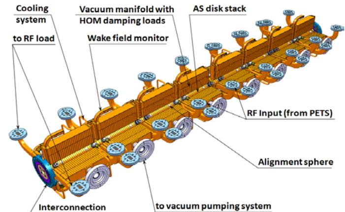
Stack of 8 ac. structures under assembly
