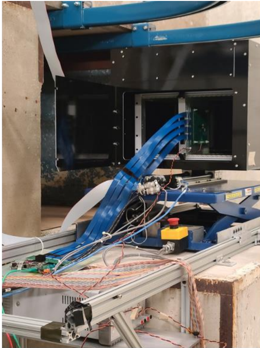
CMS ECON-T ASIC irradiation. Photo courtesy D. Noonan (FNAL).
