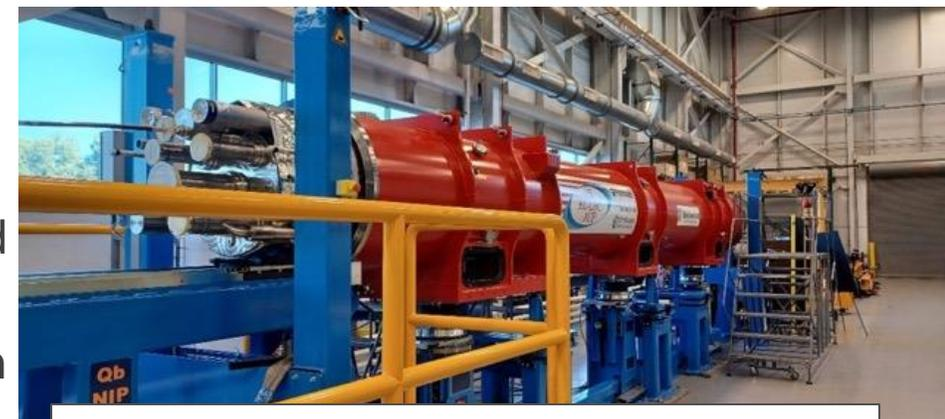
Q1/Q3 Cryo-assembly with two 4.2m long Magnets
