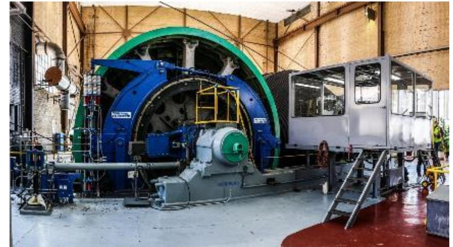
In March 2021, contractors completed major mechanical and electrical upgrades to the Ross Hoists at SURF (originally manufactured in the 1930s). Ross Hoists will power the excavation of 800 Ktons of waste rock and serve as the conveyance for people, materials and equipment underground.
