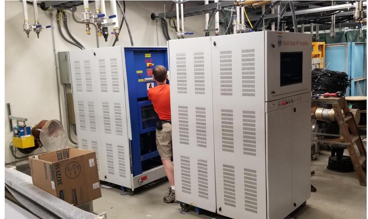
RRCAT 40 kW 650 MHz prototype amplifiers under testing at Fermilab. Will power 650 MHz cryomodule testing at PIP2IT
