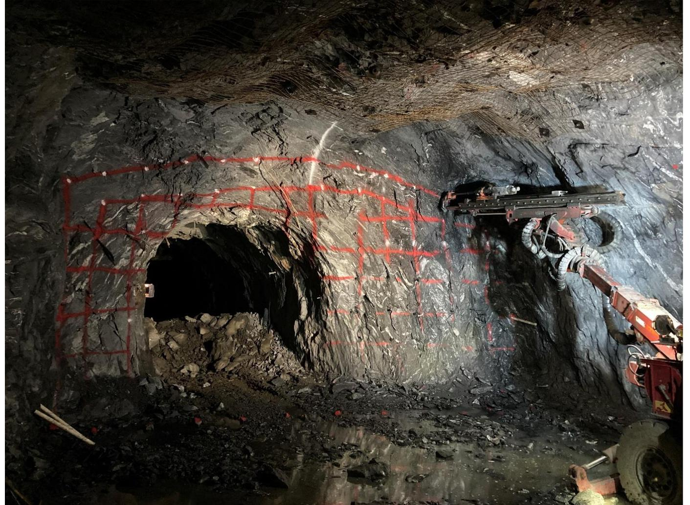
Drilling Charge Holes in the 4850-81 Face
