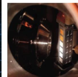
ATES sensor mounted at the SLAC X-ray synchrotron.
