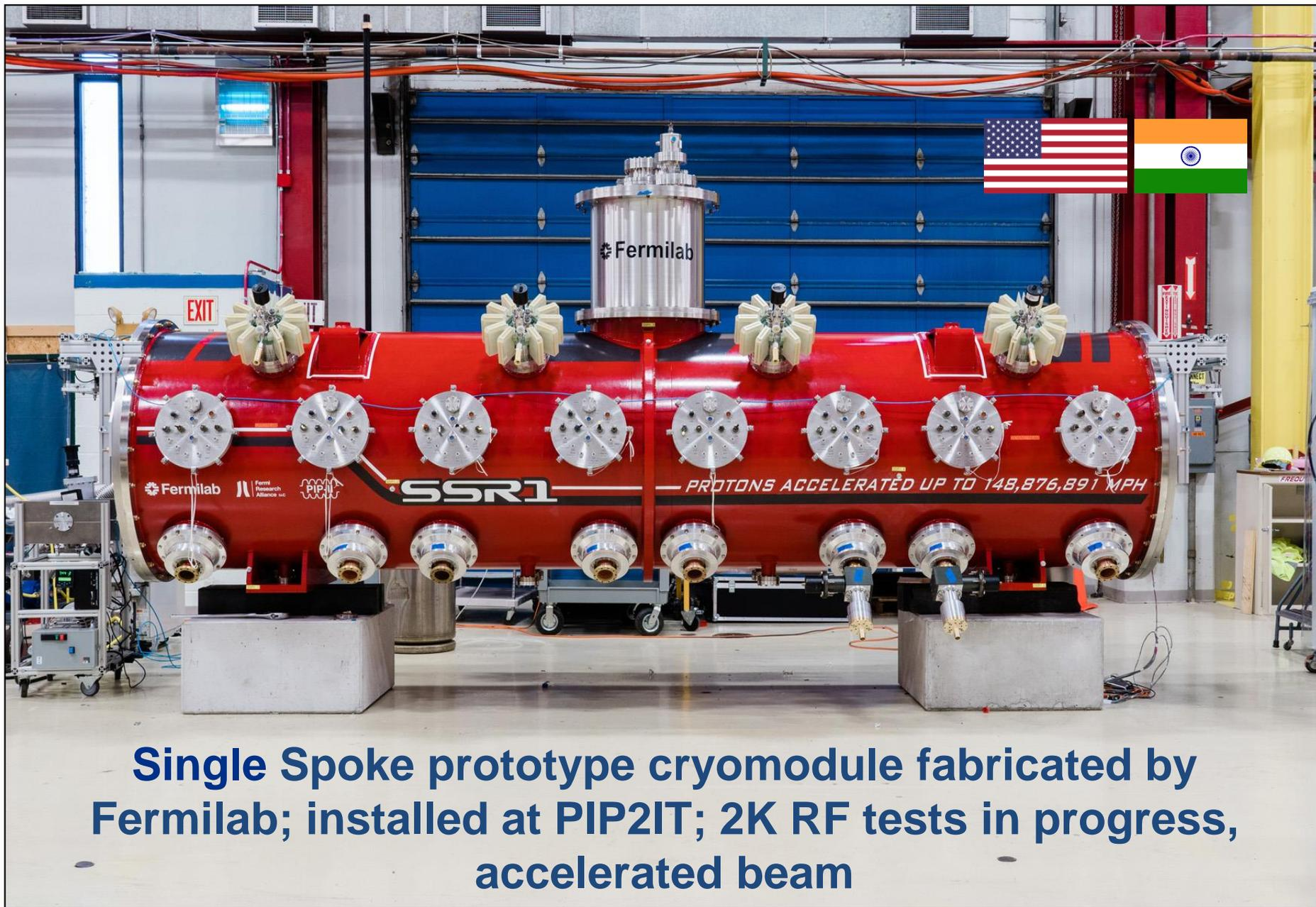
**Single Spoke prototype cryomodule fabricated by Fermilab; installed at PIP2IT; 2K RF tests in progress, accelerated beam**
