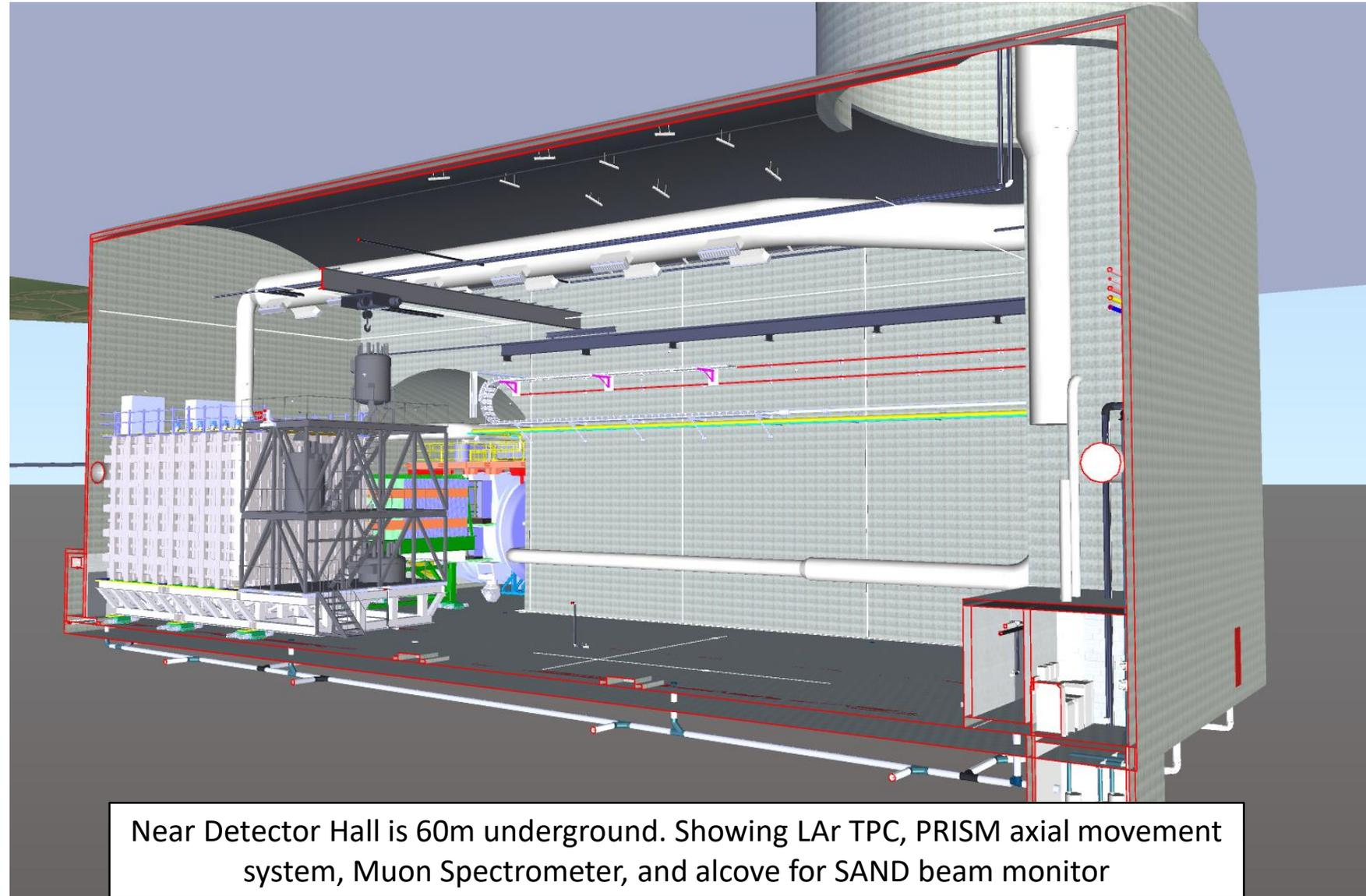
Near Detector Hall is 60m underground. Showing LAr TPC, PRISM axial movement system, Muon Spectrometer, and alcove for SAND beam monitor
