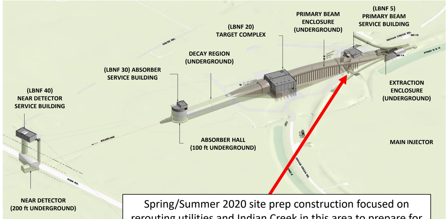
Spring/Summer 2020 site prep construction focused on rerouting utilities and Indian Creek in this area to prepare for the main LBNF construction planned to begin Fall 2023
