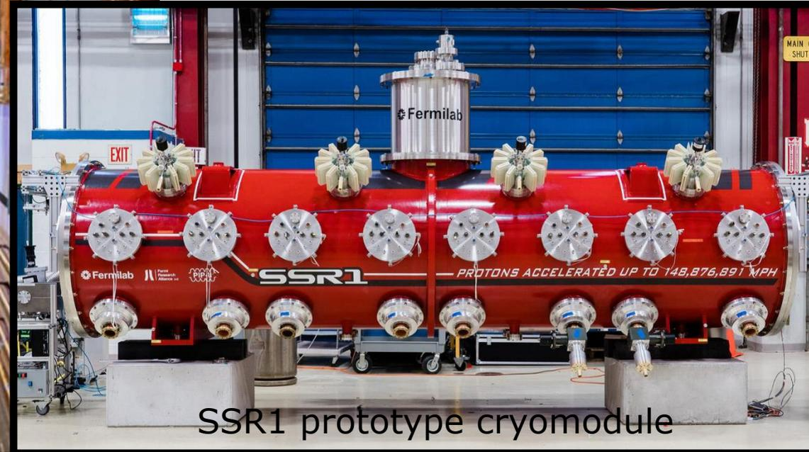
SSR1 prototype cryomodule
