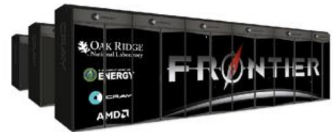
*The exascale systems Aurora (Argonne) and Frontier (Oak Ridge) expected in the 2021/22 timeframe; both systems are >1EF, ~10PB system memory, >200PB file systems at ~10TB/s. One cabinet is roughly 10PF; both systems are CPU/GPU (compute dominated by the GPUs)*
