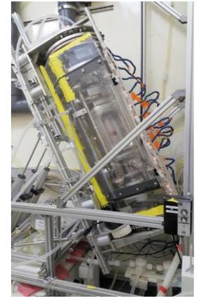
Rotational BCP tool for RFD cavity (ANL/FNAL facility)
