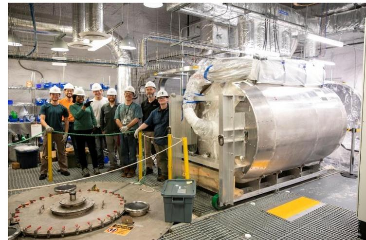
LZ TPC inside ICV after transport underground at SURF on Oct 21, 2019
