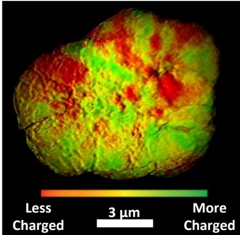
Compositional heterogeneity in a  $\text{LiNi}_{1/3}\text{Co}_{1/3}\text{Mn}_{1/3}\text{O}_2$  battery after hundreds of hours charging
