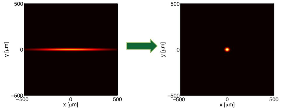
Comparison of the beam profiles of ALS (left) and ALS-U (right).
