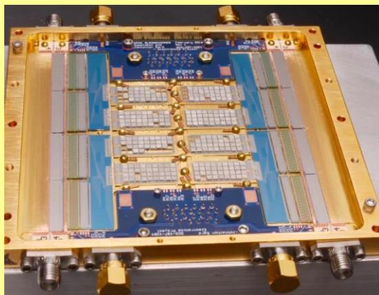
**Fast, high-efficiency superconducting X-ray detector**
