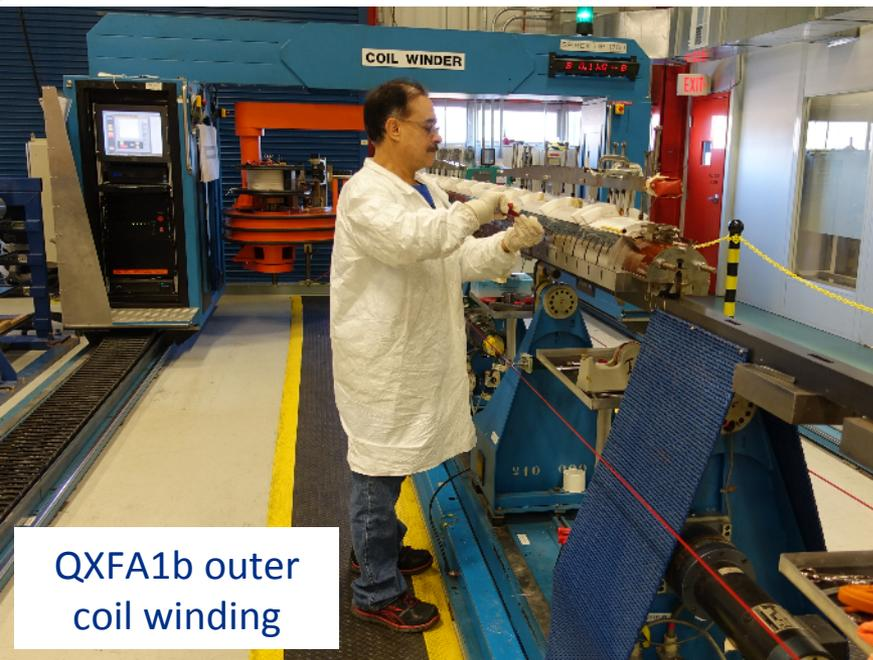
QXFA1b outer coil winding
