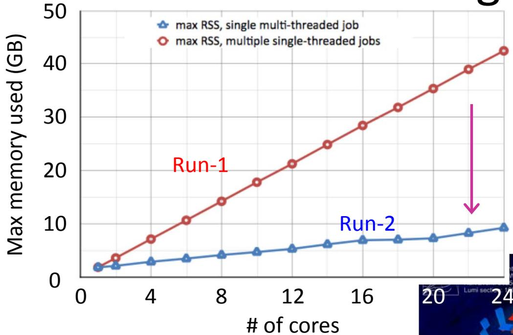
Updating to a multi-threaded framework reduces memory footprint needed to reconstruct events
