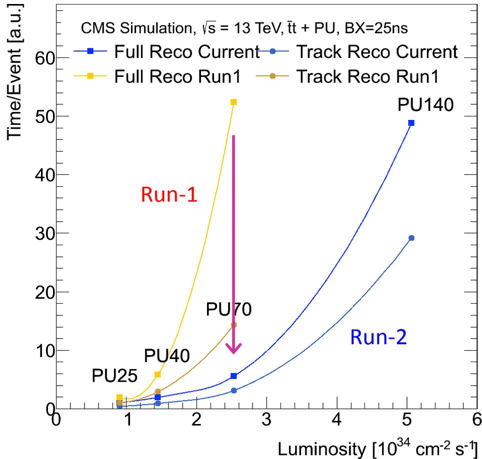
Updates to event reconstruction reduces processing time to manageable levels in a high pileup environment
