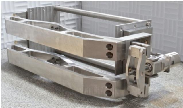
Double-Lever tuner prototype
