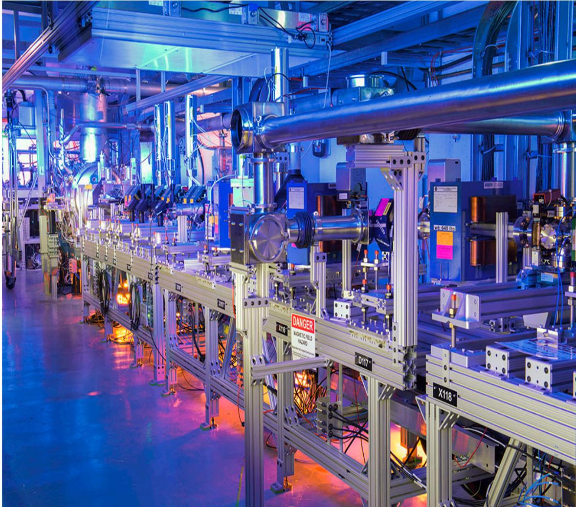
On Friday morning, March 27 first beam was delivered. We were able to deliver a 20 MeV electron beam from the IOTA-Injector photocathode, through a 1 m long SRF booster cavity CC2, and all the way to the beam dump, in front of the SRF Cryomodule 2.
