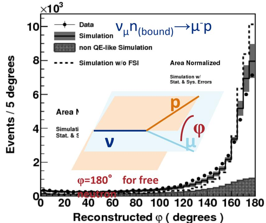
Phi is the angle between the neutrino-muon and neutrino-proton planes. If the original neutron that is struck is free and at rest, then phi is always 180 degrees. Clearly there is more happening inside the nucleus than that and these data are the first to measure this reaction from the final state proton side.
