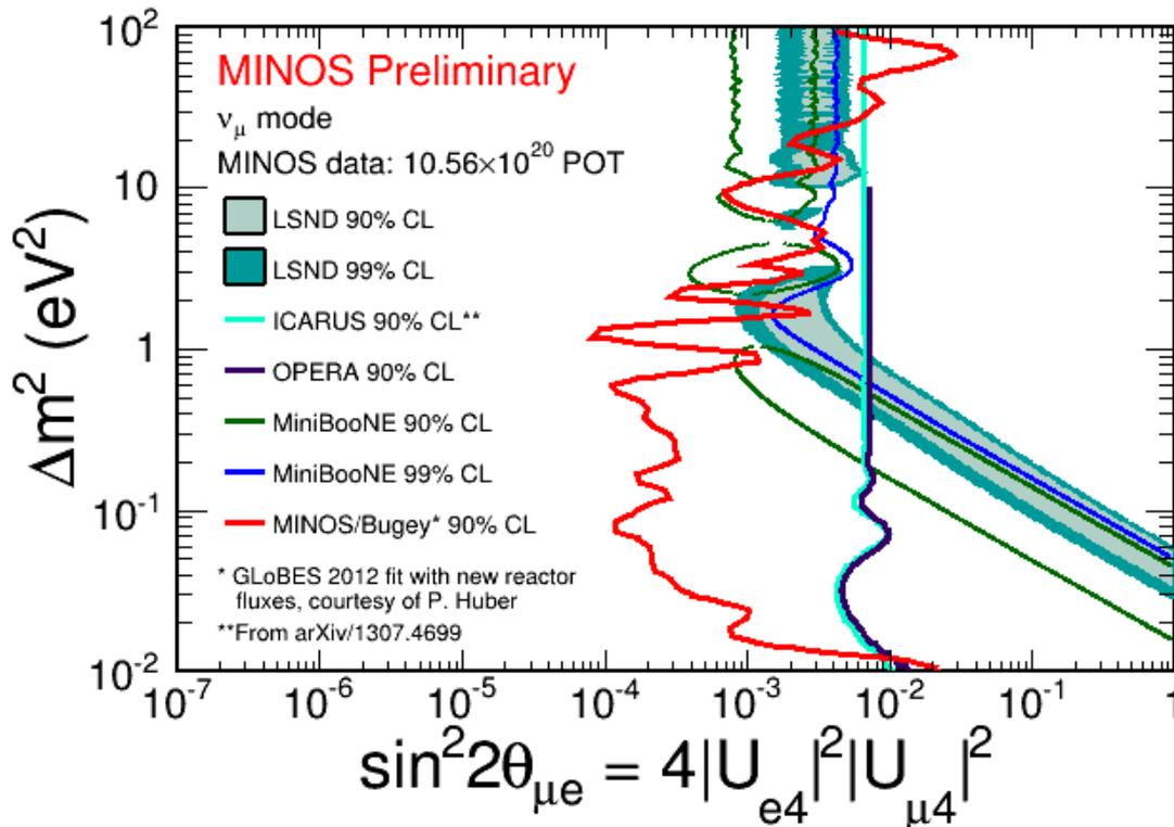
Combining MINOS NC and CC disappearance data with  $\nu_e$  disappearance data from the Bugey Reactor gives combined limits that can be compared to MiniBooNE, LSND, ICARUS, and OPERA results
