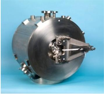
First SSR1 prototype with prototype tuner for HINS (2010)
