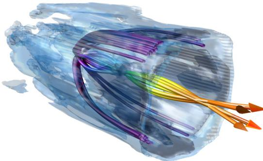
*Figure 1.* Computer simulation shows electrons being trapped and accelerated in a “bubble” (blue-grey cup-like structure) from a laser wakefield accelerator. Particle tracks are also shown for electrons successfully trapped by the wake. The color of the tracks, from purple to red, shows the increase in electron energy along the track. (Image: W.B. Mori and L.O. Silva)
