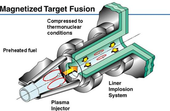
a) The 10-microsecond variant of MIF utilizes the magnetic pressure produced by a 12-MA current to implode a cylindrical metallic liner (green). A magnetically confined plasma formed outside the liner (red ellipses to the left of liner) is injected into the liner as it is imploding. This plasma is compressed and heated to fusion conditions by the time the imploding liner stagnates against the plasma. (AFRL/LANL collaboration)
