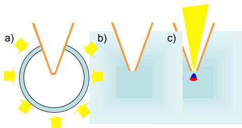
*Figure 1.* a) In a fast-ignition target, the outer shell (blue) is irradiated by a compression driver (yellow) to b) create a dense fuel core, which is then c) ignited by a picosecond laser (yellow) to create electrons (blue). The electrons propagate into the dense core and create an ignition spark (red).
