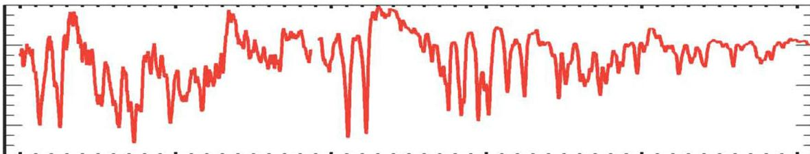
Figure 2. Transmitted intensity versus wavelength - transmission spectrum for iron heated to 1.8 million degrees. The peaks and valleys of the data carry a wealth of information about the different electronic states iron atoms take in the plasma, such as in the interior of a star. This type of data can be used to test quantum mechanical models of iron opacity.
