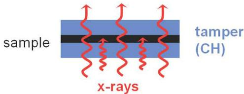
Figure 1. X-rays stream through a sample and heat it uniformly over its volume. Uniformity is key because it enables comparison with models for X-ray transmission that assume a single temperature and density throughout the material. Transmission is measured by positioning an X-ray source below the sample and recording the transmission spectrum, an example of which is shown in figure 2, with a spectrometer positioned above the sample.
