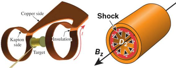
b) In this one-nanosecond variant of MIF, a target containing fusion fuel is contained in a cylindrical tube (labeled “target”). A magnetic field is applied along the axis of the cylinder by the copper coil, and the target is then imploded by laser ablation. A shock wave launched into the fuel ionizes and heats it, and the target implosion compresses the plasma to fusion conditions. (LLE, Univ. of Rochester)
