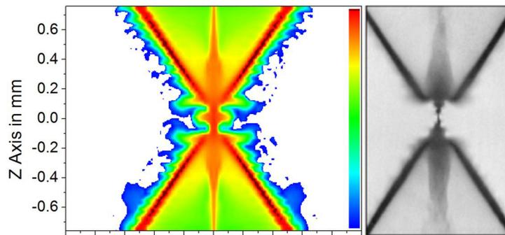
*Figure 2.* At left, a slice through a 3-D simulation of an imploding X-pinch reveals the formation of a narrow plasma column where the wires cross. At right, a flash of X-rays from one X-pinch (not shown) is used to capture the instant when the center of a second X-pinch collapses to a few millionths of a meter. (Left image, Imperial College; right image, Cornell University)
