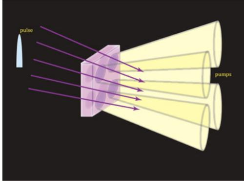
*Figure 2.* Relatively long pulses of laser light (yellow), not necessarily tightly focused, irradiate the plasma slab (purple) from the right. A counter-propagating short pulse of light (arrows) differing from the other by the frequency of the electron plasma waves can then capture the energy of the longer pulse and remain focused. (Image: N.J. Fisch and V.M. Malkin)
