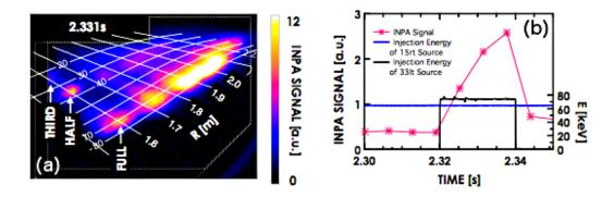
FIG. 16: (a) INPA image across a co-current, nearly-tangential NB blip for DIII-D discharge #173110. (f) Symbols show the time evolution of the integrated signal over the phosphor image. Timing of the background (blue) and active (black) NB sources is shown by solid lines. (Adapted from Ref. [48]).
