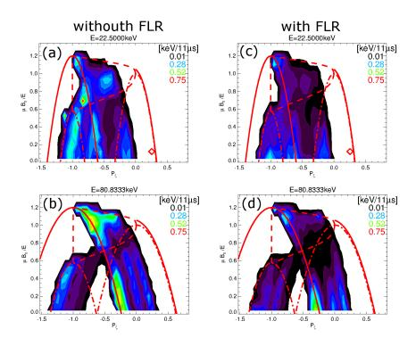
FIG. 38: Average energy kicks in phase space at two representative fast ion energies computed for a TAE transport probability matricx from ORBIT. Left column: FLR corrections are neglected in ORBIT. Right column: FLR corrections are included.
