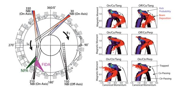
FIG. 24: Left: elevation of DIII-D showing the injection geometry for the available NB sources. Right figures show typical deposition locations in phase space (red symbols). Contours represent the root-mean-square energy kicks from NTM instabilities. (Adapted from Ref. [63]).
