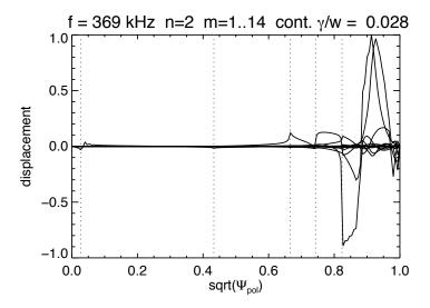
FIG. 11: Displacement  $\xi$  vs. flux surface function  $\sqrt{\Psi_{pol}}$  of the mode at f=369 KHz from NOVA-K calculation. Input parameters are from t=930 ms of the plasma shown in Fig. 10.
