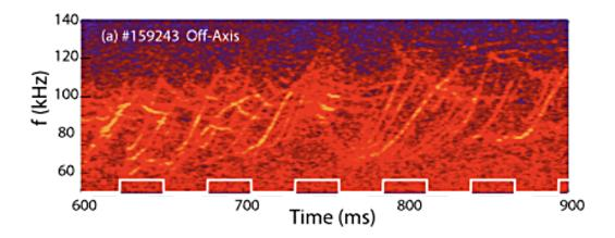
FIG. 1: Spectrum from the cross-power of two CO2 interferometer chords for DIII-D discharge #159243. The color scale is logarithmic in the amplitude. Waveform for a modulated NB source is shown as a white line. Coherent activity below 50 kHz and above 140 kHz is negligible. (Adapted from Ref. [7]).
