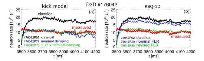
FIG. 31: Neutron rate predictions from (a) kick model and (b) RBQ-1D models. Measured neutron rate is shown in red. Classical predictions are shown in black.
