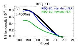
FIG. 33: Fast ion density profiles at t = 4000 ms from TRANSP simulations with enhanced fast ion transport via (a) kick model and (b) RBQ-1D.
