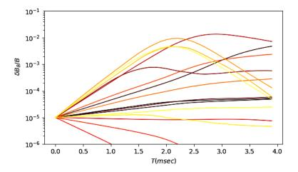
FIG. 28: RBQ-1D self-consistent evolution of 11 Alfvénic modes, including RSAE and TAE modes. The time around t=2 ms, at which the larger-amplitude modes are near saturation, corresponds to the time used to evaluate the diffusion coefficients of beam ions. Stable modes whose amplitude decays in time can be identified and removed from further analysis.
