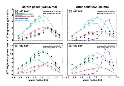
FIG. 36: Comparison of experimental FIDA brightness profile vs the profile reconstructed through FIDASIM for kick and RBQ-1D model results. In the anomalous diffusion model, an anomalous fast ion diffusivity of  $D_b \sim 3.5 \text{ m}^2/\text{s}$  was used to match the measured neutron rate.
