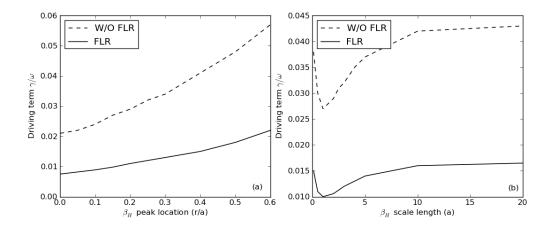
FIG. 14:  $\beta_H$  peak location and scale length scan for the driving term. (a)  $\gamma_{drive}/\omega$  vs.  $\beta_H$  peak location both with FLR and without FLR. (b)  $\gamma_{drive}/\omega$  vs.  $\beta_H$  scale length both with FLR and without FLR.
