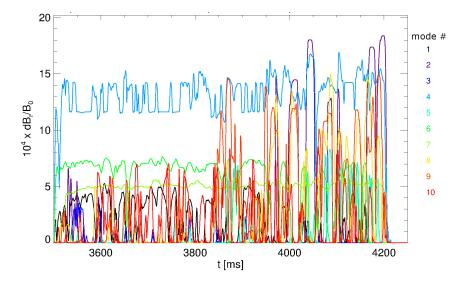
FIG. 27: Saturated amplitude as a function of time computed through the kick model in TRANSP for 16 Alfvénic modes. Some of the curves represent the joint evolution of multiple modes.
