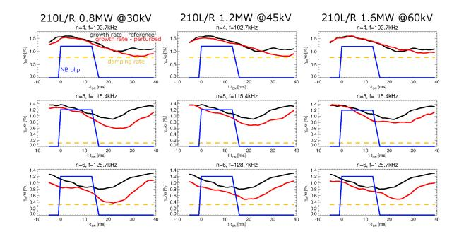
FIG. 20: TRANSP/kick model exploration of using modulation of the counter-current NB sources to mitigate or suppress RSAE/TAE instabilities. The three columns refer to different assumptions on the NB injection voltage and power. For each setting, linear growth rates  $\gamma_{lin}$  are shown for three modes. Modulated NB waveform (blue) and damping rate (yellow) from NOVA-K are shown as reference. Modes would be stabilized for  $\gamma_{lin}$  below the yellow line.
