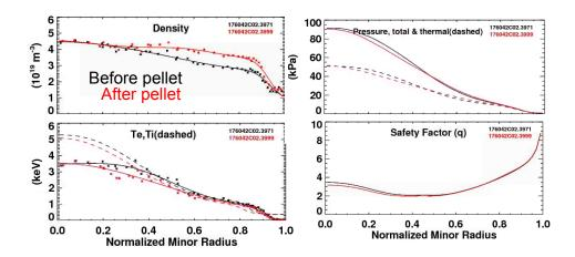
FIG. 21: Profiles of density, temperature, pressure and safety factor around t = 4000 ms for DIII-D #176042.
