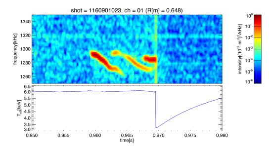
FIG. 15: TAE mode observed in 3-ion ICRF heating experiment (shot 1160901023) on Alcator C-Mod. Top: Spectra from PCI density fluctuations vs. frequency and time. Bottom: time trace of  $T_{e0}$
