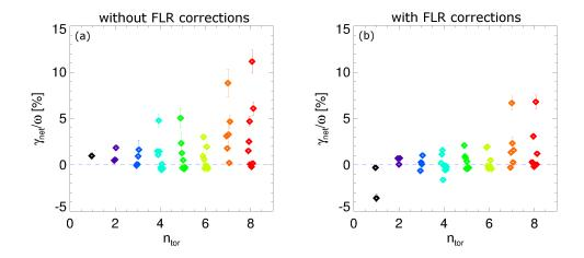
FIG. 25: Net linear AE growth rate from kick model stability analysis for DIII-D #176042. Colors identify different toroidal mode numbers. (a) Computed rates neglecting finite Larmor radius (FLR) effects. (b) Rates computed with a simplified model to include FLR effects in the ORBIT gyro-center code. The computed reduction in growth rate is more significant as the toroidal mode number increase and modes structures become more localized.
