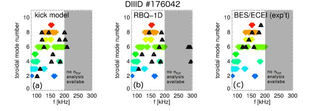
FIG. 29: Comparison of measured toroidal mode number spectrum as a function of frequency (colored symbols are used to differentiate different mode numbers) with predicted spectrum from (a) kick model and (b) RBQ-1D linear analyses, shown as black symbols. (c) Black symbols show frequency and mode number of modes for which a good match between NOVA-K eigenmodes and experimental data from BES is obtained. Only (linearly) unstable modes are shown for the kick and RBQ-1D predictions.
