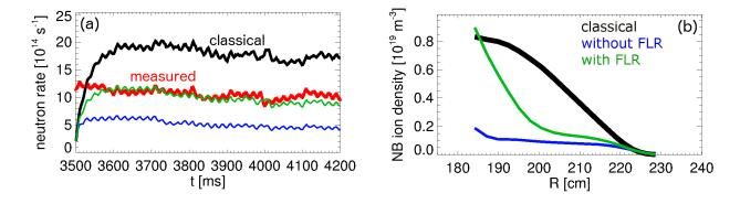
FIG. 37: (a) Neutron rate from kick simulations using the nominal mode amplitudes inferred from the experiment. Blue curves refer to simulations for which FLR corrections are not included to compute the transport probability matrices. Green curves are obtained by including FLR corrections. Measured and classical neutron rates are shown for comparison. (b) Corresponding NB ion density profiles at t = 4000 ms.
