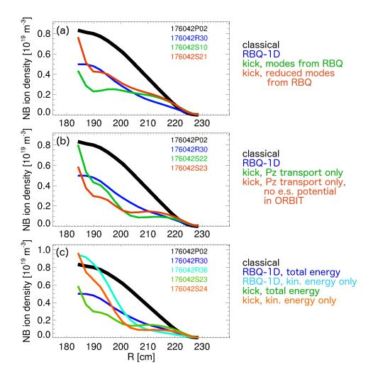
FIG. 40: Benchmark simulations between kick and RBQ-1D models. The kick model transport probability matrices are modified to mimic the main RBQ-1D assumptions in terms of number of harmonics retained in the model, transport in  $P_{\zeta}$  only and negligible electrostatic potential and rotation.
