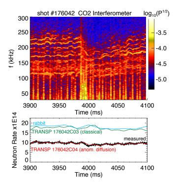
FIG. 22: Top: spectrum of density fluctuations measured through interferometry for DIII-D discharge #176042. The change in the observed fluctuations around t = 4000 ms is caused by injection of a large pellet that modifies plasma density and temperature. Bottom: neutron rate from TRANSP and from the RABBIT code [60].
