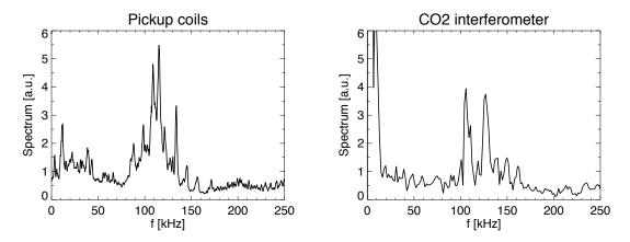
FIG. 30: (a) Magnetic fluctuation spectrum from Mirnov coils. (b) Density fluctuations from a vertical interferometer chord intersecting the mid-plane around mid-radius.
