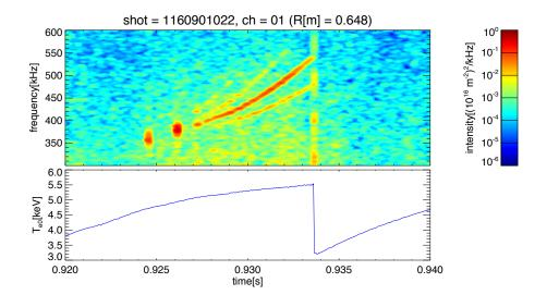
FIG. 10: TAE mode observed in 3-ion ICRF heating experiment (shot 1160901022) on Alcator C-Mod. Top: Spectra from PCI density fluctuations vs. frequency and time; Bottom: Time trace of  $T_{e0}$ .
