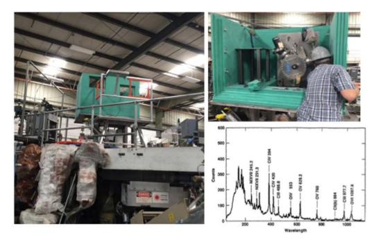
Figure 12. During the third quarter, most of the Divertor SPRED assembly was installed on DIII-D, including the neutron shielding. Commissioning was nearly completed in the fourth quarter, just as the FY17 DIII-D run time target was achieved. The system will be ready for operations in November, 2017. Expected spectra shown at lower right.
