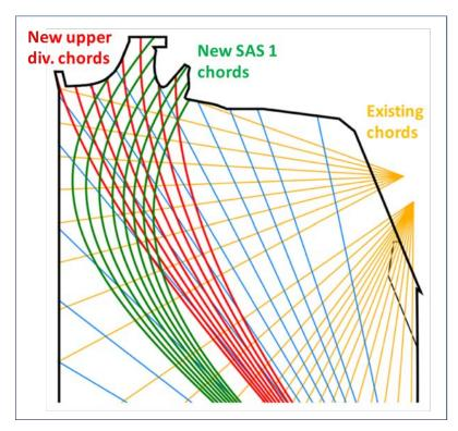
Figure 7. New tangential viewing chords in the upper divertor (red) and SAS divertor (green) will enable bolometer measurements of total radiated power in these closed configurations.
