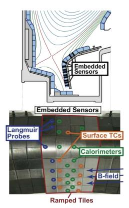
Figure 47. Location of surface thermcouple sensor array (Surface TCs) in a 'ramped tile' outer divertor module.
