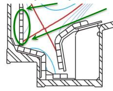
Figure 33. Cross-section of C-Mod's lower closed divertor, showing the vertical inner target. The IR camera views the target within the green circle along sight-lines that angle down from the right (green arrows).
