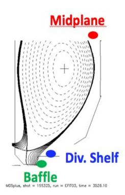
Figure 23. A schematic of the NSTX-like shape and gas injector locations that were used to study detachment similarities.
