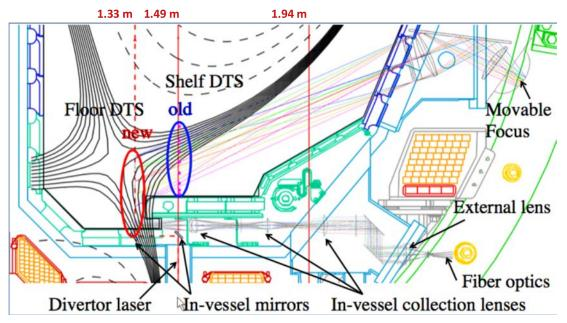
Figure 14. In-vessel mirrors permit use of the DTS laser at R=1.33 m on the lower floor (circled in red). This new capability enables high-fidelity electron density and temperature measurements for a much wider range of divertor geometries.
