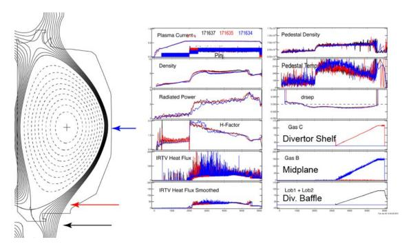
Figure 1. The NSTX-U plasma shape in DIII-D. Three gas puff locations used for divertor detachment were compared in these three shots. In contrast to NSTX-U results, the plasma conditions on DIII-D (in the NSTX-U shape) are not sensitive to the location of the gas puff used for detachment. This is consistent with previous DIII-D results in lower triangularity plasmas.
