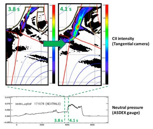
Figure 9. In Shot 171578, the divertor radiation front, as visualized by a tangential camera filtered for CII emissions (top), moves away from the upper ceiling, signaling detachment onset. This event coincides with a sharp increase in divertor neutral pressures as measured by the ASDEX gauge (bottom). This correlation points to ASDEX gauges as a promising diagnostic for registering detachment in closed divertors with limited spectroscopic views.
