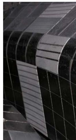
Figure 21. Outer divertor ‘Rail probe’ array consists of 21 flush-mounted probes, toroidally extended and aligned with the pitch of the local magnetic field.
