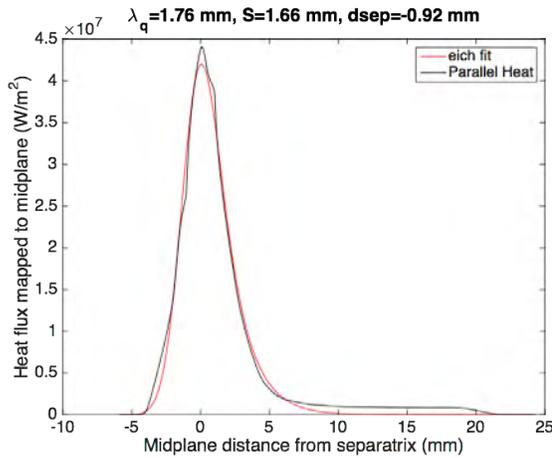
Fig. 7. Heat-flux footprint mapped back to outside midplane on the 1.5MA DIII-D discharge #144981. The Eich formula yields an excellent fit, with  $\lambda_q^{XGC1} \approx 1.8$ mm.
