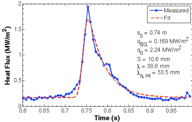
**Fig. 42. Experimental divertor heat-flux footprint for the lowest current NSTX shot #132368 with  $I_p = 0.7$ MA and  $B_{pol} = 0.2$ T. This figure is different from other experimental footprint figures in that it is plotted at the divertor plates and not mapped back to the outboard midplane. Thus, the numbers shown in this figure are not to be compared with other numbers presented in this report.**
