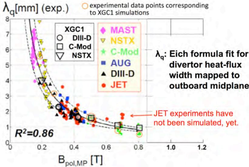
**Fig. 43. Simulation data overlaid on Eich’s experimental data set [Eich2013]. The solid line represents Eich’s  $1/B_{pol}^{1.19}$  regression formula.**
