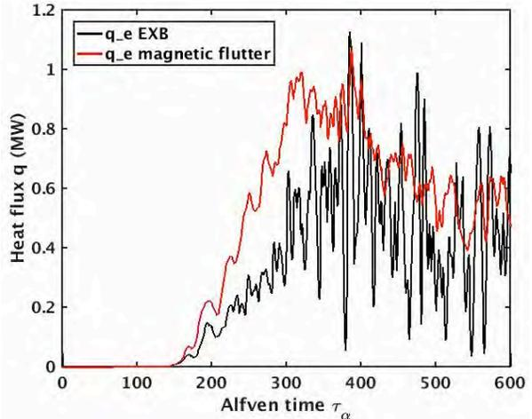
Fig.5 time trace of the magnetic flutter-induced radial energy transport (red curve) and E×B drift induced radial energy transport (black curve) across the separatrix
