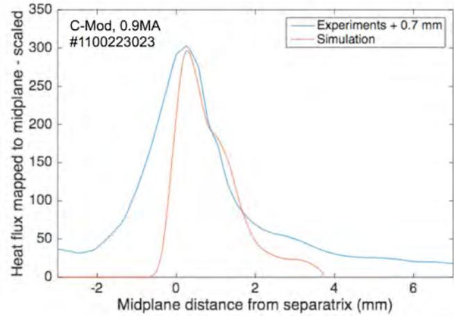
Fig. 18. XGC1 footprint (orange) does not show a large spreading into the private flux region, as seen in the experimental infrared profile (blue), while the outward e-folding length agrees well.
