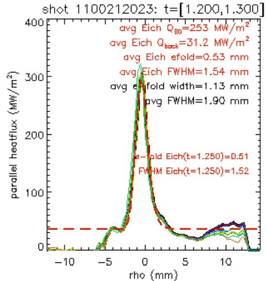
Fig. 17. Experimental heat-flux footprint analysis for C-Mod #1100223023.
