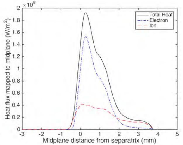
Fig. 21. Electron contribution from turbulence effect is dominant over ions contribution in the 0.9MA C-Mod simulation.
