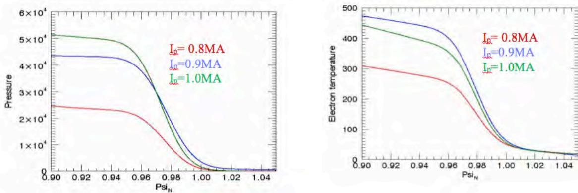
Figure 28. Profiles of total pressure (left) from kinetic EFIT g-file, electron temperature (right) in pedestal region of C-Mod EDA H-mode, linearly extrapolated into the SOL.
