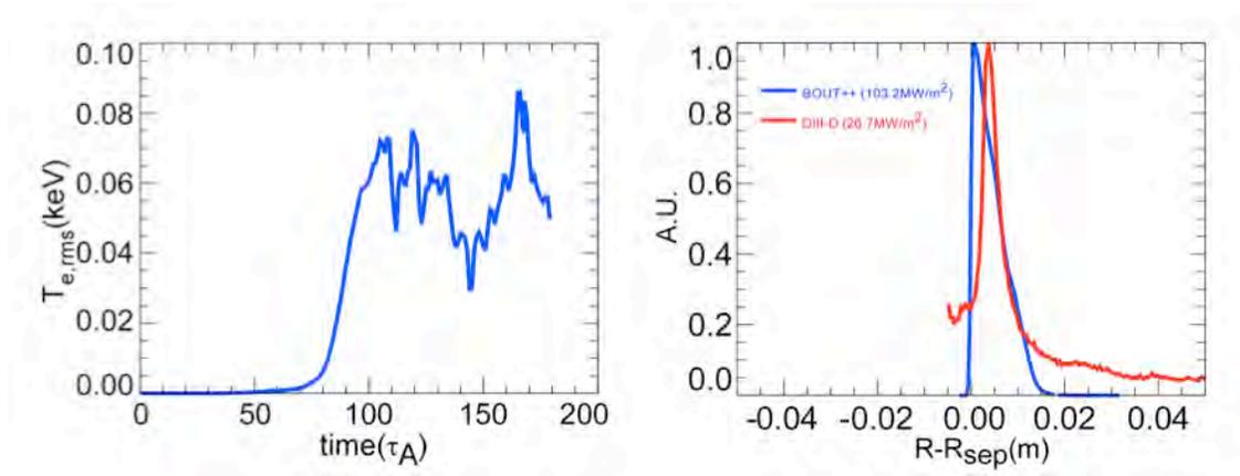
Figure 27. (left) BOUT++ time history of the rms amplitude of electron temperature fluctuation at outside midplane for discharge 144977 with current  $I_p=1\text{ MA}$ : (right) Radial profile of parallel heat flux mapped to the outer midplane for DIII-D IR-inferred heat flux measurement at outer divertor target (Red), and from BOUT++ simulation (time averaged) at the outer divertor target (Blue). All the parallel heat flux profiles are *normalized by the corresponding maximum values*.
