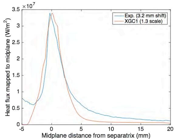
Fig. 8. Heat-flux footprint shape comparison between XGC1 (divided by 1.3) and experiment (moved inward by 3mm) on DIII-D discharge #144981.
