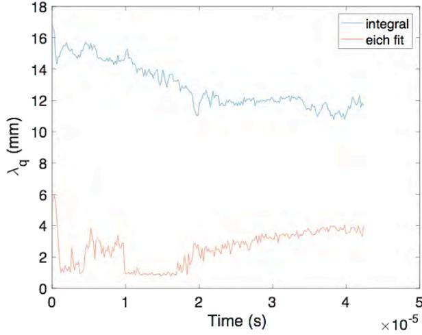
**Fig. 41. Quick saturation of  $\lambda_q$  after  $t \sim 0.03$ ms in this lowest poloidal field XGC1 simulation of NSTX shot #132368 ( $I_p = 0.7$ MA,  $B_{pol} = 0.2$ T).**
