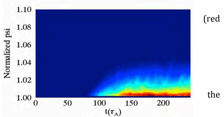
Fig. 2 Contour plot of divertor parallel electron heat flux versus normalized poloidal flux and time from BOUT++
