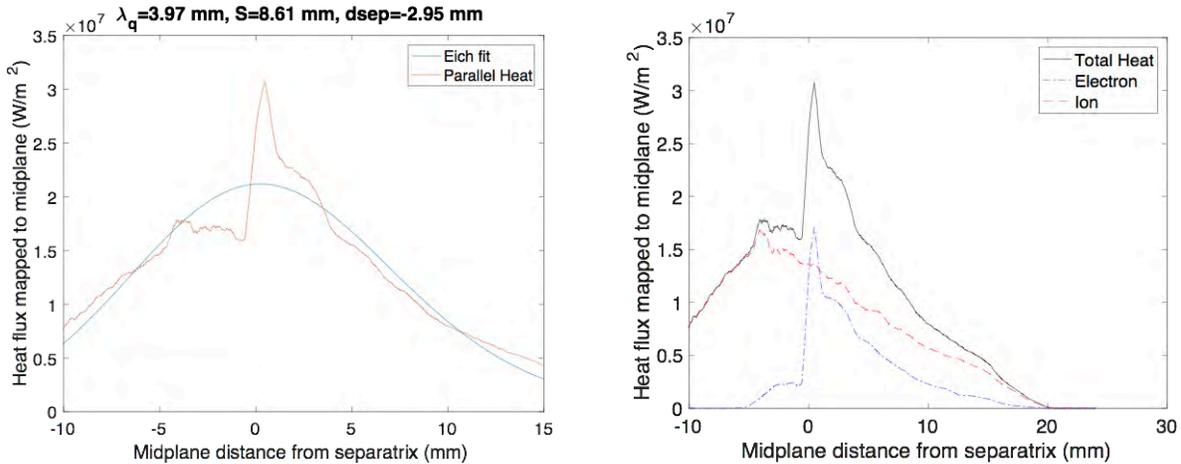
**Fig. 40. (left) The XGC1 simulated divertor heat flux profile, showing a significant spread into the private flux region. (right) Decomposition of the heat flux profile into ion and electron contributions, without considering the strong neutral particle effect near the divertor plates, shows that the excessive spreading into the private flux region is caused by the ions.**
