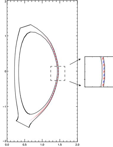
Figure 8. Linear eigenmode structure for toroidal mode number  $n=100$  for the high current  $I_p=1.13$  MA NSTX discharge #128797 using the diamagnetic stabilization model.
