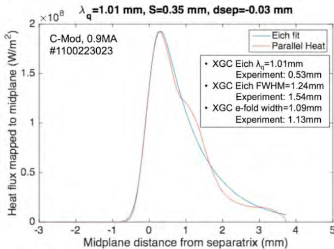
Fig. 16. Divertor heat-flux footprint, mapped back to outboard midplane as calculated by XGC1 for the higher current C-Mod discharge #1100223023.
