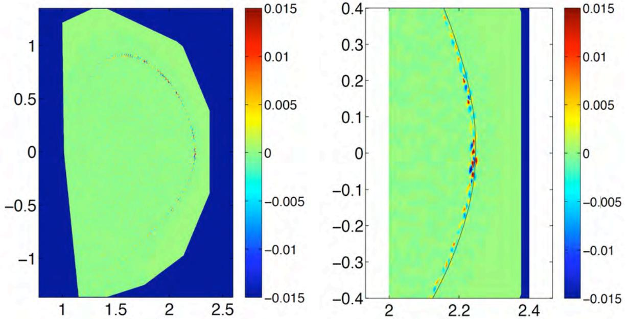
*Fig. 4a (left). Initial growth of the normalized density perturbation from a nonlinear simulation in XGC1-particle just inside the magnetic separatrix for the 1.5MA DIII-D case. Fig. 4b (right). Enlargement of the region around the outboard midplane. Penetration of the “blobs” outside of the magnetic separatrix (black curve) is already visual at the outboard midplane.*
