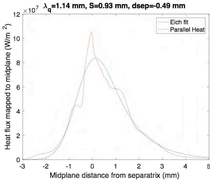
**Fig. 33. Diverter heat flux footprint for C-Mod shot #1100223012, 0.8MA, simulated by XGCI (red line) and the corresponding Eich formula fit (blue)**
