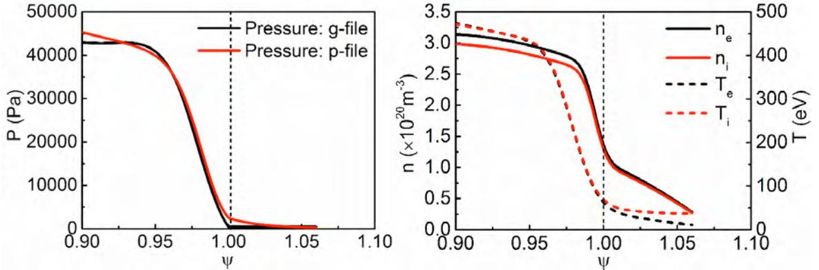
Fig. 10. Profile of (left) total pressure from kinetic EFIT g-file and from measurements in p-file, and (right) electron density and temperatures in pedestal region of C-Mod EDA H-mode #1100212023.
