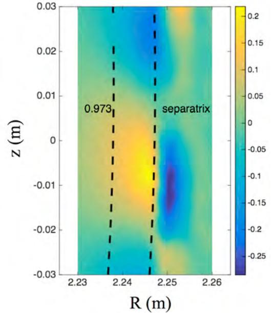
Fig. 6. Nonlinear blobby turbulent  $\delta n/n$  from XGC1, measured at outboard midplane from the DIII-D 144981 simulation.
