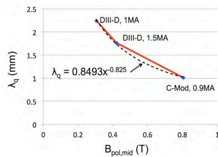
Fig. 13. XGC1 simulation results of the Eich heat-flux width  $\lambda_q$  from three different data points over two different tokamaks. Both the magnitude and the  $B_{pol}^{-\gamma}$  trend of  $\lambda_q$  agree qualitatively well with the experimental database shown in Fig. 14.
