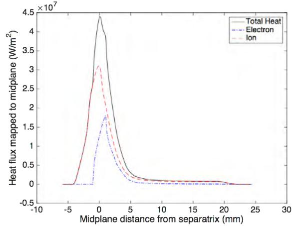
Fig. 9. Comparison of the heat-flux footprint between ions and electrons in the same DIII-D discharge as in Figs. 6-8.
