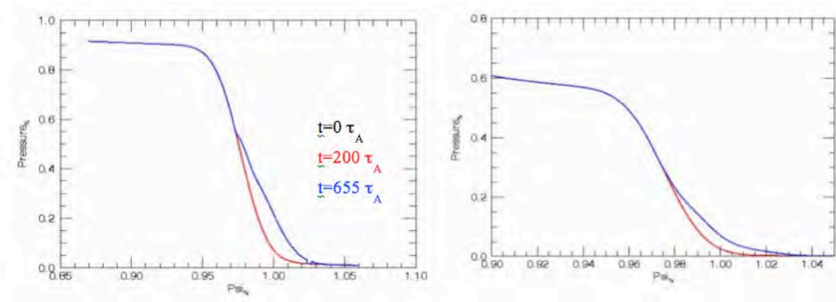
Figure 30. The pressure profiles at outside midplane at different times for discharge 11002120023 (left) with current  $I_p = 0.9$  MA and 1100223012 (right) with  $I_p = 0.8$  MA.
