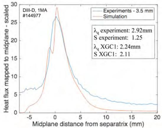
Fig. 24. Comparison of the divertor heat-flux footprint between experiment and XGC1 for the DIII-D 1MA discharge
