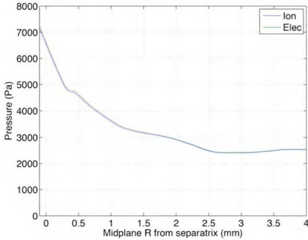
Fig. 20. Upstream electron and ion pressure profile at outboard midplane in the 0.9MA C-Mode simulation, as observed in XGC1.
