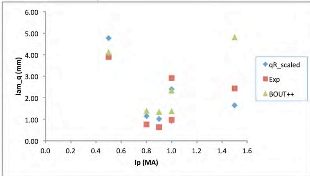
Figure 11 Comparison of  $\lambda_q$  vs  $I_p$  for the discharges simulated with BOUT++ showing the experimental measurement (Exp), the simulation result (BOUT++) and the scaling from a simple theoretical estimate ( $qR_{\text{scaled}}$ ) that is roughly proportional to the connection length.
