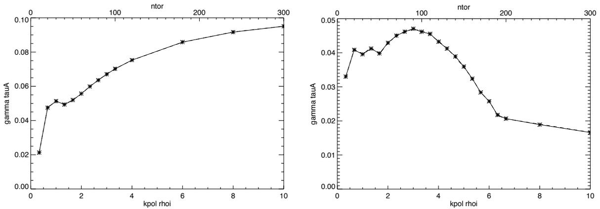
Figure 32. Linear growth rates for the high current  $I_p=1.0$  MA NSTX discharge #128797: (a) resistive ballooning mode model, (b) diamagnetic stabilization model of the vorticity equation.
