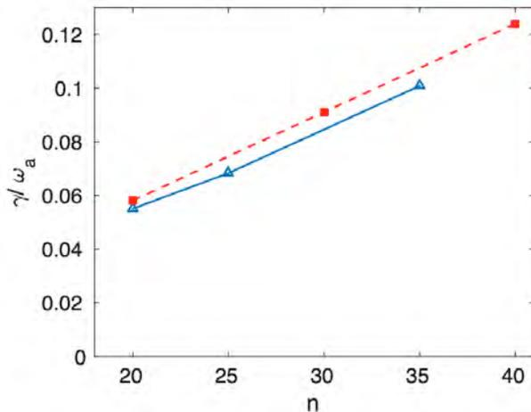
*Fig. 5. Cross verification of the electromagnetic modes between XGC1 (blue) and BOUT++ (red) for intermediate to high toroidal mode number  $n$  modes. DIII-D discharge at 1.5MA is used.*
