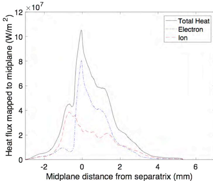
**Fig. 36. The width of the simulated electron heat flux in C-Mod shot #1100223012 is comparable to that of the total and greater than that of the ion heat flux, indicating that blobby turbulence is playing a significant role.**
