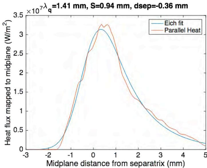
**Fig. 37. Divertor heat flux footprint for the XGC1 simulation of the C-Mod low current (0.5MA) shot #1100223026 (red line) and the associated Eich formula fit (blue).**
