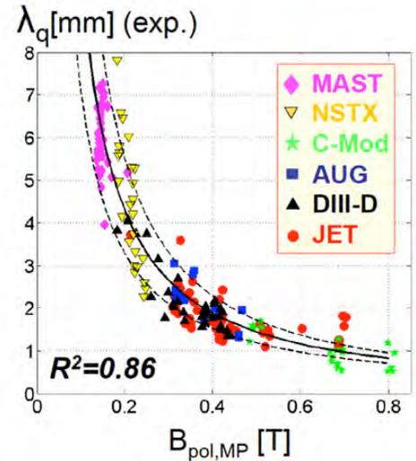
Fig. 14. The trend  $\lambda_q \propto B_{pol}^{-\gamma}$  seen from experimental data on existing tokamaks.  $\gamma$  is on the order unity. [T. Eich, Nucl. Fusion, 2013]
