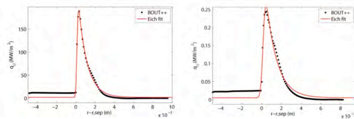
Figure 31. The profiles of parallel divertor heat fluxes for discharge 11002120023 (left) with current  $I_p = 0.9$  MA, and 1100223012 (right) with  $I_p = 0.8$  MA.
