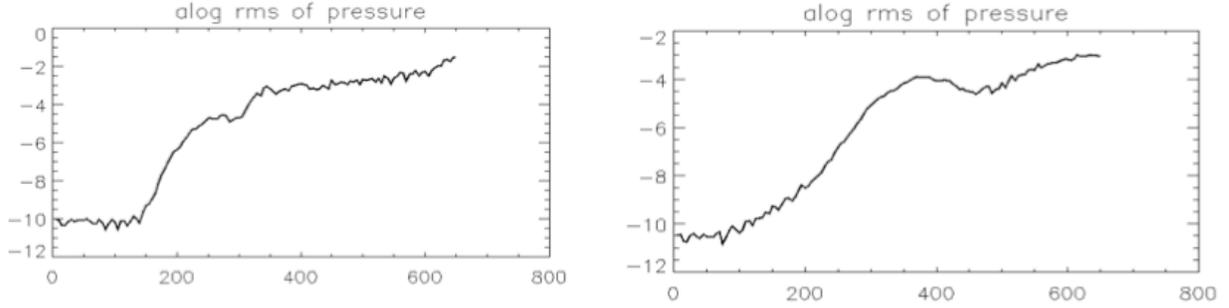
Figure 29. The time history of rms amplitude of pressure fluctuation at outside midplane for discharge 11002120023 (left) with current  $I_p=0.9\text{ MA}$  and 1100223012 (right) with current  $I_p=0.8\text{ MA}$ .
