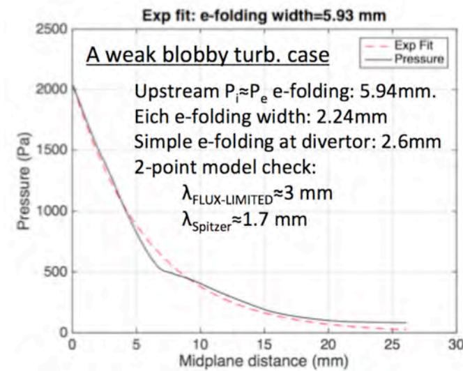
Fig. 25. Test of the two different popular 2-point models using the XGC1 data on 1MA DIII-D plasma.
