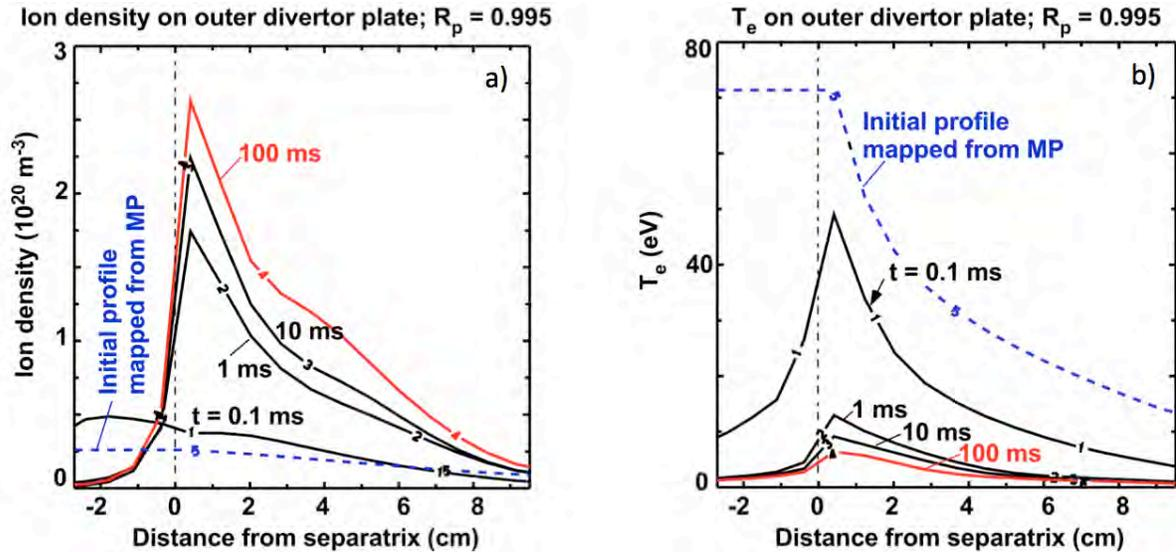
Fig. 9 Plasma density (a) and electron temperature (b) on the divertor plate for a UEDGE transport simulation initialized with poloidally constant SOL profiles and reduced neutral density at  $t=0$  sec. Initial profiles in blue and final in red.
