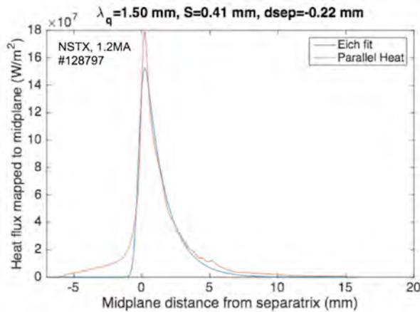
Fig. 26a. Fitting of the XGC1 data from the NSTX 1.2MA discharge simulation to the Eich formula.
