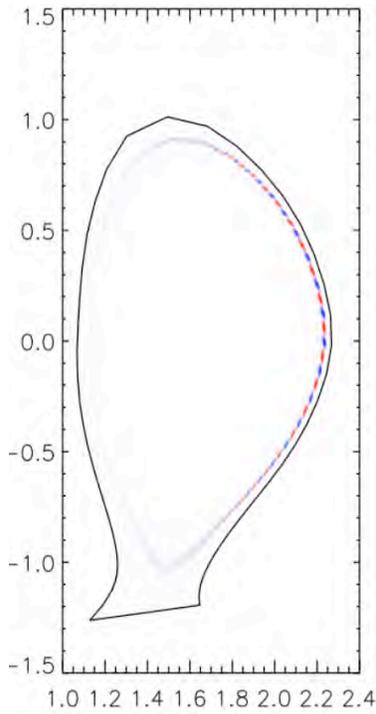
Fig. 1. Poloidal slice through the high current DIII-D H-mode discharge 144981 from BOUT++ in single-null divertor, showing pressure perturbation for dominant toroidal mode number  $n=30$  with the characteristics of the ballooning modes.
