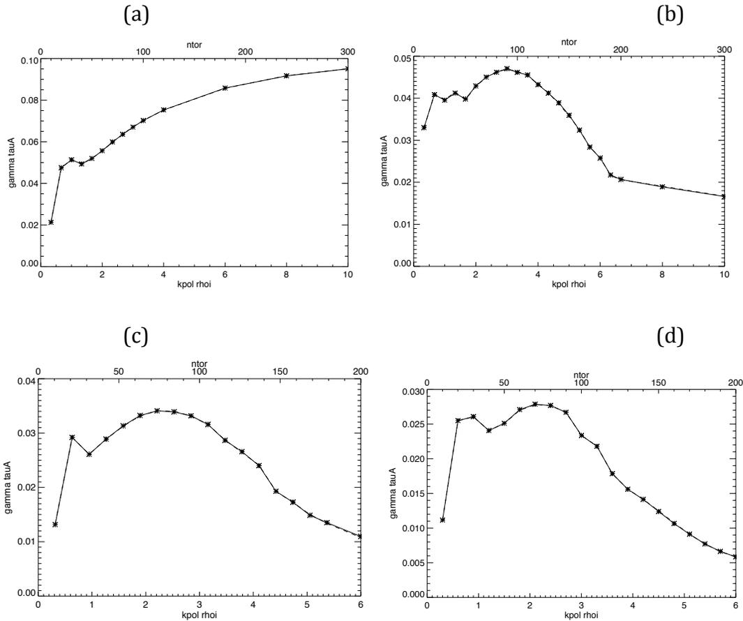
Figure 7. Linear growth rates for the high current  $I_p=1.13$  MA NSTX discharge #128797: (a) using the resistive ballooning mode model, (b) using the diamagnetic stabilization model for the vorticity equation. (c) Adding ad hoc damping near the outer boundaries tames the numerical instabilities that arise at low  $n$ , although the peak growth rate is reduced by 30%. (d) Adding ad hoc damping near the inner boundary reduces the peak growth rate by an additional 10%.
