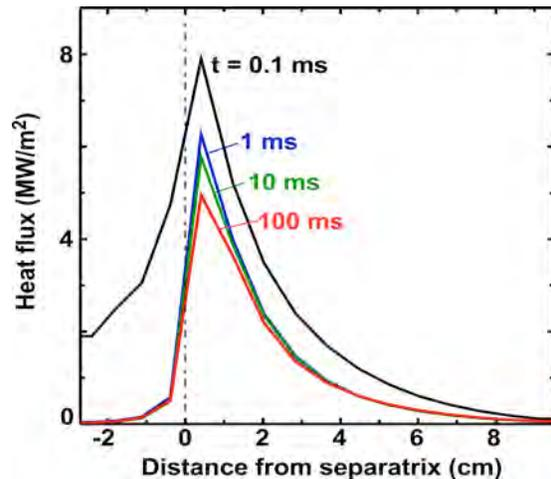
Fig. 10 Heat-flux profiles on the outer divertor plate at various times for conditions and times of the simulations in Fig. 9.
