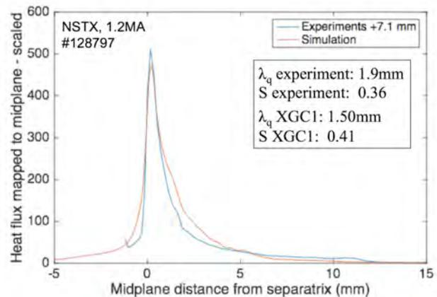
Fig. 26b. Comparison between the XGC1 footprint and the IR camera footprint for the NSTX 1.2MA discharge. The agreement is quite
