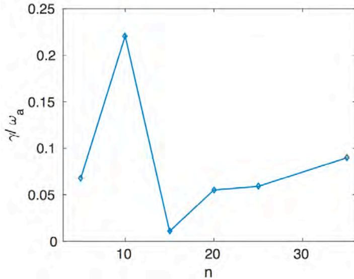
Fig. 3. Toroidal mode number ( $n$ ) spectrum in the high current DIII-D discharge (144981) from the hybrid electromagnetic calculation in XGC1-particle. Low to intermediate  $n$ -numbers are plotted here from XGC1-particle, while intermediate to high  $n$ -numbers are plotted in Fig. 2 from BOUT++. In the overlapping intermediate  $n$ -numbers ( $n=20-35$ ), the growth rates from two codes are similar.
