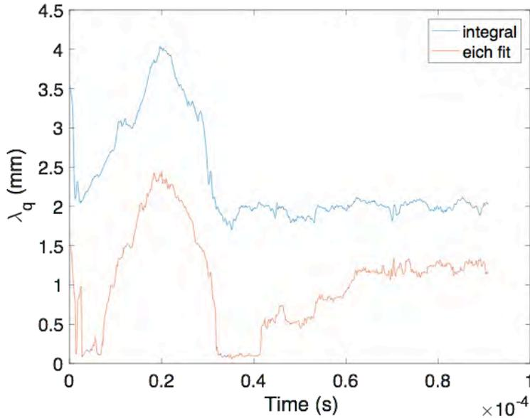
**Fig. 35. Saturation of  $\lambda_q$  in the XGC1 simulation after 0.06ms for C-Mod shot #1100223012**
