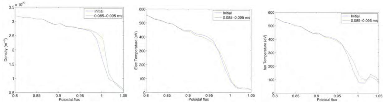
Fig. 15. Plasma profiles in the edge region of C-Mod discharge #1100223023 at 0.9MA ( $n_e$ ,  $T_e$ , and  $T_i$  from left to right). Blue lines are the inputs to XGC1, which are somewhat arbitrary at  $\Psi_N \gtrsim 1$  as explained by BOUT++ section in Q2, and the green lines are the edge profiles found by XGC1.
