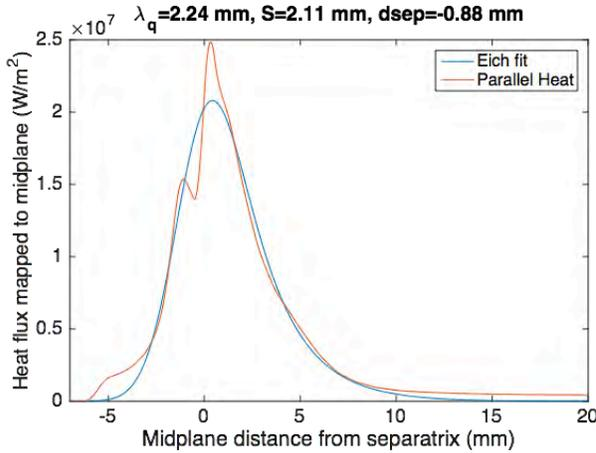
Fig. 23. Eich formula fitting of the divertor heat-flux width for the DIII-D 1MA discharge #14497.
