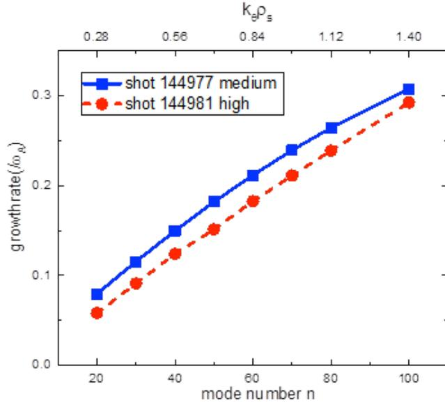
Fig. 2. Toroidal mode spectrum of two DIII-D discharges as calculated by BOUT++ for the following cases: Red for high current and Blue for medium current. The growth rates are normalized to the Alfvén frequency  $\omega_A=2.3416 \times 10^6/s$
