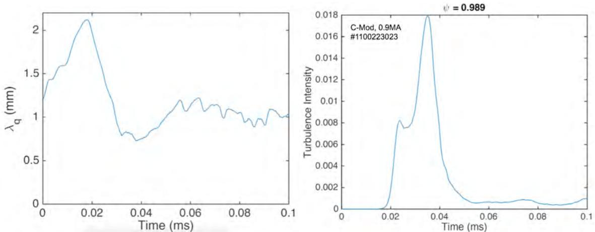
Fig. 19. Saturation of  $\lambda_q$  (left) and turbulence intensity  $(\delta n/n)^2$  (right). Turbulence intensity is plotted at  $\Psi_N \approx 0.99$  where most of the blobs are born.
