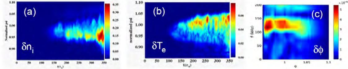
Fig. 1 (a) Ion density fluctuation; (b) Electron temperature fluctuation; (c) spectrogram vs radius
