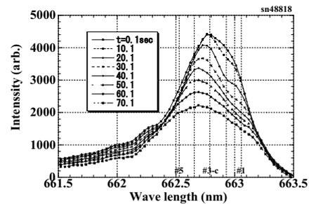
Fig.2 Temporal profile for full energy beam component for 74 s long pulse injection(sn48818).
