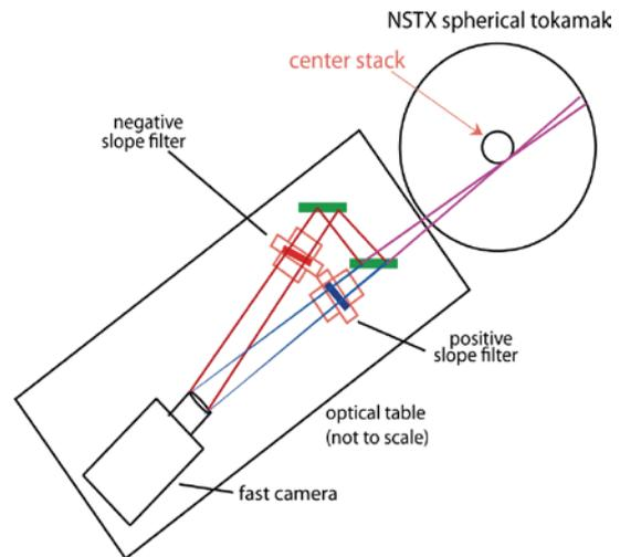
Fig. 2. Proto-type of SWIFT installed in NSTX
