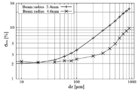
Fig. 2. The rms nonuniformity versus the pellet displacement  $dz$  in a reactor chamber for the beam radius of 3.4 mm and 4.6 mm, a pellet of the Al layer structure, the external pellet radius of 4.0 mm and the 32 HIBs system.  $\Delta\theta = 2$  degree.
