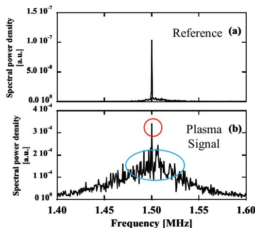
Fig. 1. Power spectrum of the reference signal (a) and that of the plasma signal of the heterodyne microwave reflectometer, during the HHFW heating in NSXT.
