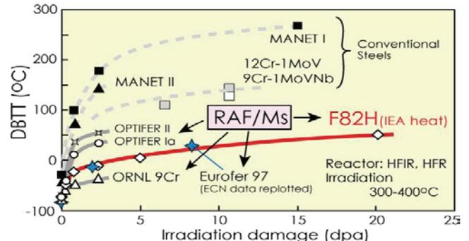
Fig.2 Damage level dependence of DBTT for F82H [2].
