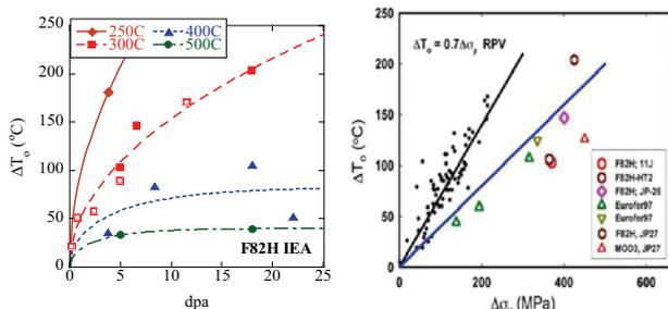
Fig. 1 a) Toughness reference temperature shift,  $\Delta T_o$ , of F82H IEA heat as a function dpa at four irradiation temperatures; b)  $\Delta T_o$  vs.  $\Delta\sigma_y$  relation for various TMS steels obtained using PCBB specimens, compared to RPV database by Sokolov et al.[1]
