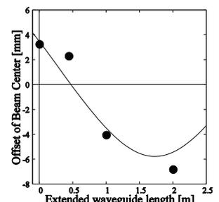
Fig.3. Dependence of offset of beam center at waveguide outlet on length of extended waveguide.
