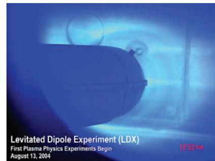
Fig.1: The floating coil and the first plasma of LDX.
