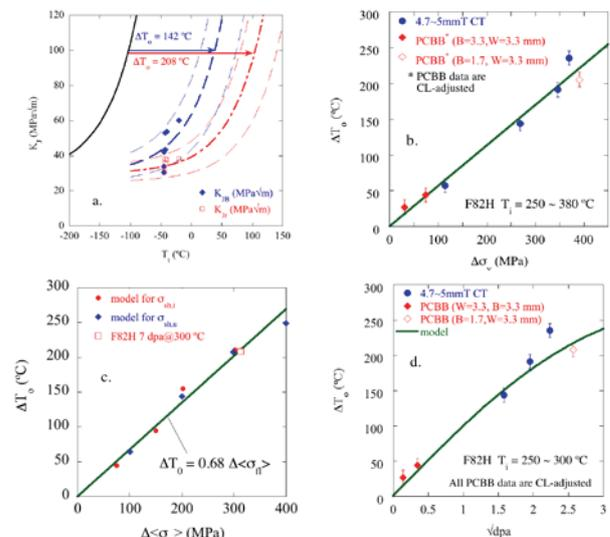
Fig. 2 a) 1T-conveted toughness data with MCs before ( $K_{JB}$ ) and after ( $K_{JR}$ ) CL adjustment; b)  $\Delta T_o$  vs.  $\Delta\sigma_y$  relations in CL-adjusted PCBB or CT specimens of irradiated F82H-IEA; c)  $\Delta T_o$  vs.  $\Delta\langle\sigma_{fl}\rangle$  (flow stress change) compared with theoretical relation study[5]; d)  $\Delta T_o$  in relatively high constraint specimens of F82H irradiated at  $\approx 300^\circ\text{C}$  with a model prediction[6].
