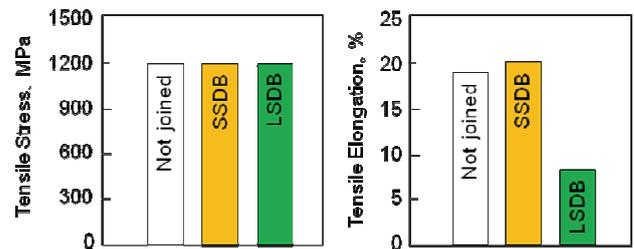
Fig.2 : Tensile stress and elongation of the ODS steel with and without joining.
