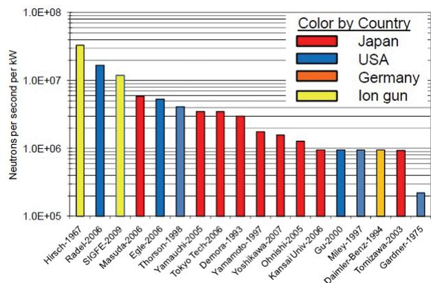
Fig.2 Neutron production rate of IEC devices<sup>1)</sup>
