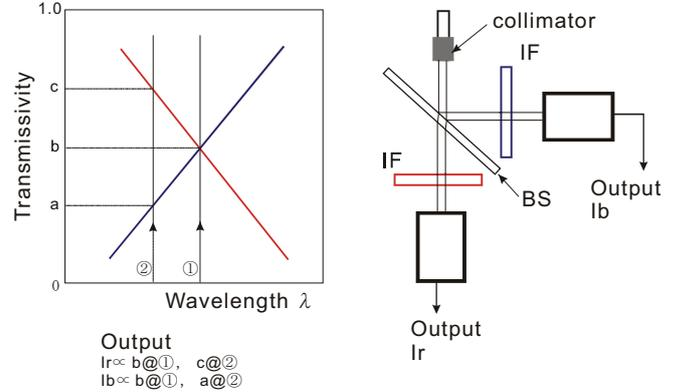
Fig. 1. Doppler shift measurement using two filters
