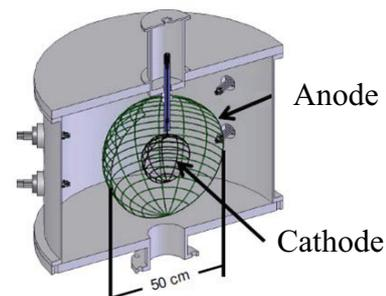
Fig.1 Schematic view of IEC device<sup>1)</sup>
