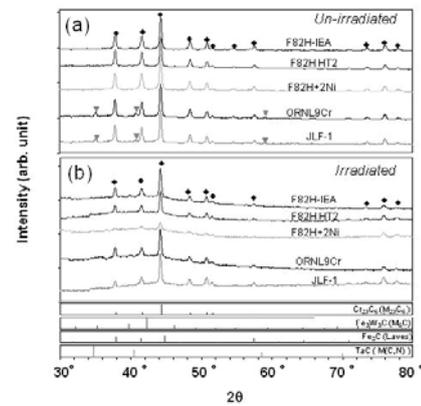
Fig. 2. XRD peaks of extracted residue from unirradiated and irradiated RAFTs. Peaks marked with diamonds correspond to the peaks from  $M_{23}C_6$ , and those marked with triangles correspond to peaks from MX (TaC).
