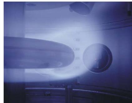
Fig.2: The floating coil and the first plasma of Mini-RT.
