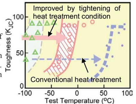
Fig.3 Improvement of DBTT-shift by tightening/optimization of heat treatment [5]. Lower postirradiation DBTT was achieved.
