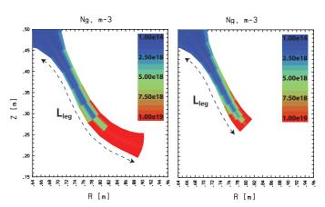
Fig. 1 – Distribution of neutral gas density is shown for the outer divertor leg, indicating the steady-state location of the detachment front. Regardless of the leg length, the detachment front location is similar for the same exhaust power.
