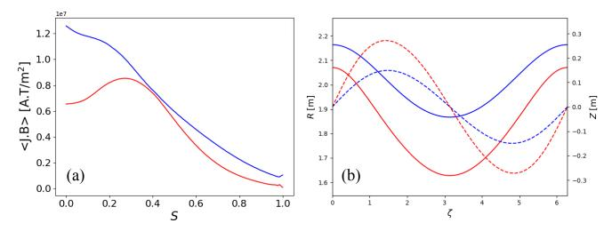
**Figure 2.** (a) The field-aligned current and (b) the magnetic axis position are shown for an initial QSH state (blue) and a case optimized for the excursion of the helical axis (blue). Both the radial (solid) and vertical (dashed) positions of the magnetic axis are shown.
