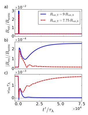
Figure 1. Comparison between a) the externally applied magnetic field  $B_{\text{ext}},$  b) the field response  $|B_{\text{res}}|,$  and c) the flow frequency at the rational surface  $\omega_{\text{res}}$  for two computations with different magnitudes of the magnetic transient  $B_{\text{ext}}.$  The effect of the larger transient is to precipitate a transition to a low-slip, field-penetrated state, while the smaller transient returns to the high-slip, flow-screened equilibrium.
