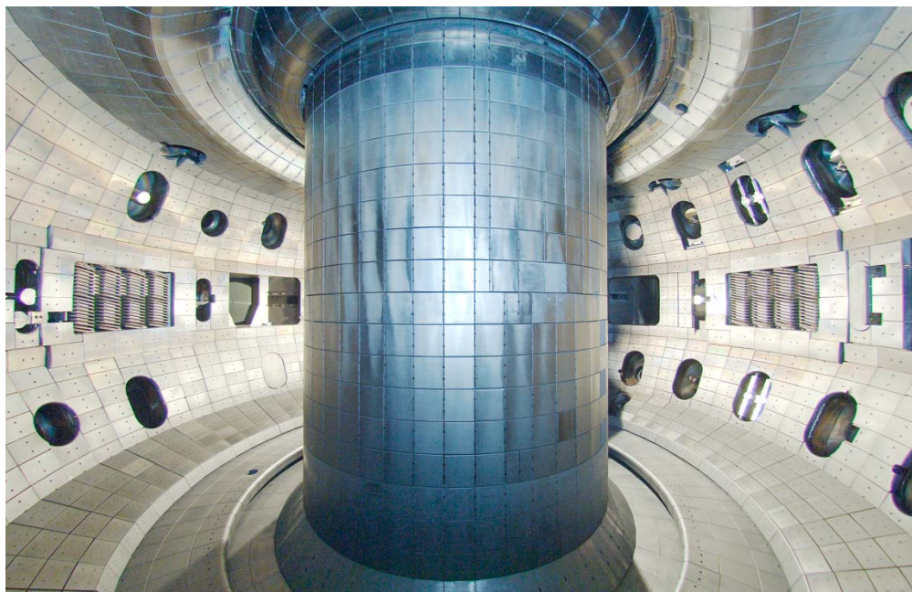
Interior of DIII-D vacuum vessel
