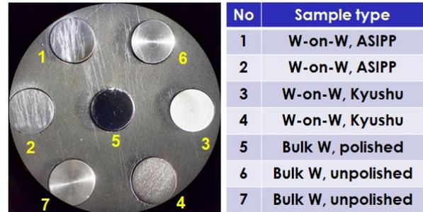
Figure 1. Post-exposure photograph of the DiMES head with sample buttons showing evidence of arcing
