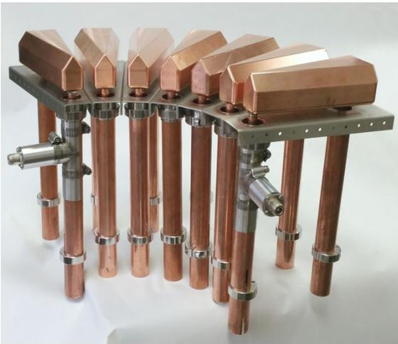
Figure 3. The radial top launch CCCL antenna, inverted.
