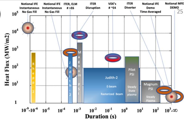
Figure 1: Landscape of heat flux and current international HHF testing devices.
