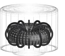
*Innovation:* Arrays of planar magnets on the surface which should offer a cheaper, lower maintenance pathway to fusion.
