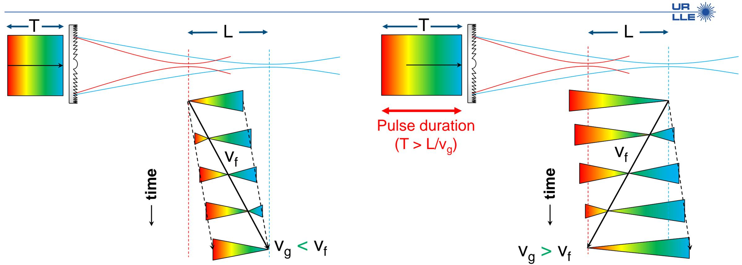
The chromatic focusing creates an extended focal range, while the chirp sets the time at which each frequency comes to its focus providing control over the velocity of the intensity peak
