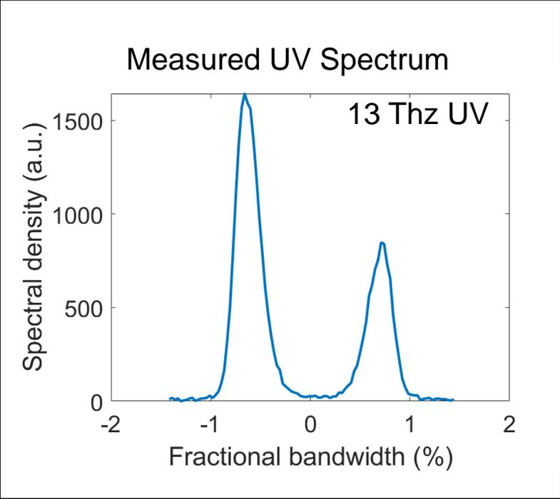
Novel concept demonstrates efficient broad band ( $\Delta\omega/\omega > 1.5\%$ ) UV frequency tripling
