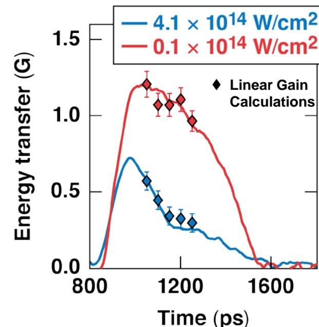
Experiments demonstrate linear CBET models used in integrated ICF simulations are robust
