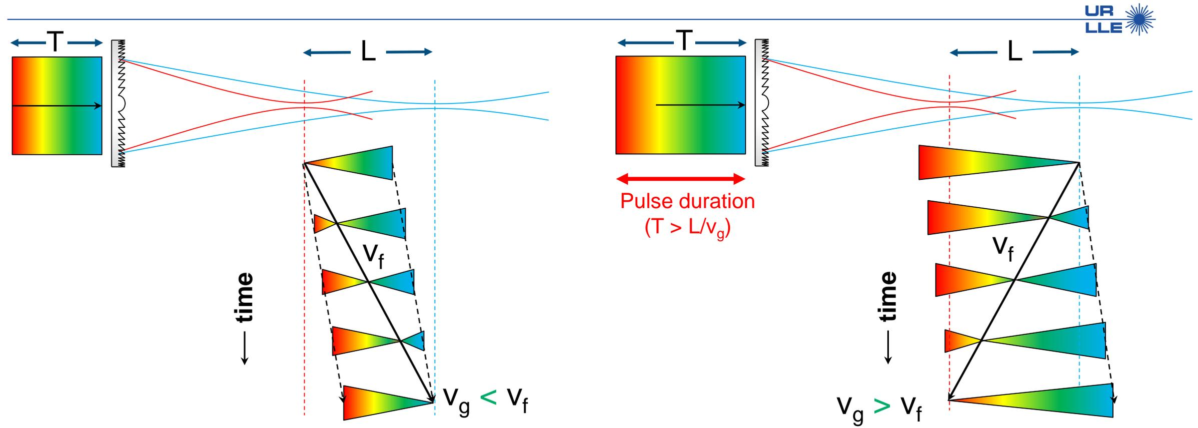
The intensity peak is propagating faster than the group velocity of light
