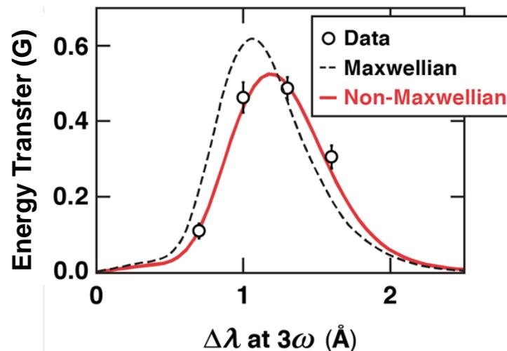
NonMaxwellian distribution functions shift the CBET resonances used to tune symmetry in hohlraum experiments on the NIF
