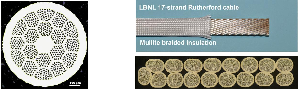
Figure 4.2.2. Bi-2212 strand cross section and Rutherford cable.
