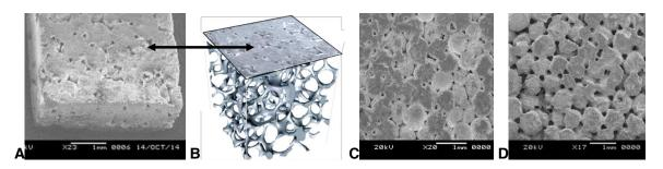
Figure 4.4.2A-D: SEM image of cellular breeder block (A), tomography scan showing network of interconnected internal micro-channels (B), and SEM images of 90% dense (C), and 78% dense (D) Li<sub>2</sub>ZrO<sub>3</sub> cellular breeder fabricated using foam skeletons having different ligament diameters.
