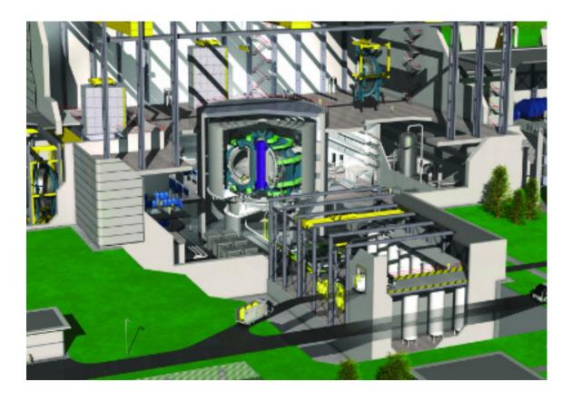
Schematic representation of the ITER plant, <u>https://www.iter.org/sci/Fusion.</u>
