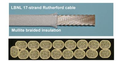
Figure 4.2.2. Bi-2212 strand cross section and Rutherford cable.
