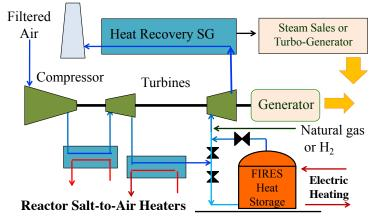
Figure 6.7.2. Nuclear air Brayton Combined Cycle with high-temperature energy storage provides high efficiency with load following.
