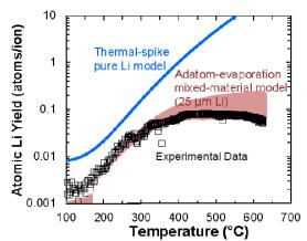
Figure 5.1. Erosion of lithium under high-flux deuterium bombardment as a function of surface temperature. The gross erosion, measured via spectroscopy, can be described with an adatom-evaporation and mixed Li-D material model that takes into account concentration-dependent hydrogen diffusivity in the bulk Li.
