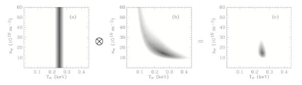
Figure 4.1.3. Probability Density Functions from a) soft X-ray data and b) Thomson scattering measurements of electron density, illustrating the combination of multiple diagnostics using a Bayesian statistical framework<sup>9, 10</sup>. The result of combining a) and b) is the reduced posterior PDF (lower uncertainty) shown in c) for the combined data.
