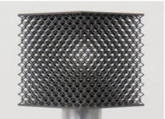
Figure 4.3.1. Rhombic dodecahedral lattice structure made of 316SS using SLM. Photo courtesy of LLNL.
