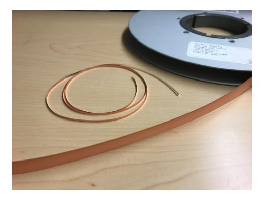
Figure 4.2.1. Two commercial tapes from SuperPower: 12 mm wide, 100  $\mu$ m thick tape and 2 mm wide, 45  $\mu$ m thick tape.
