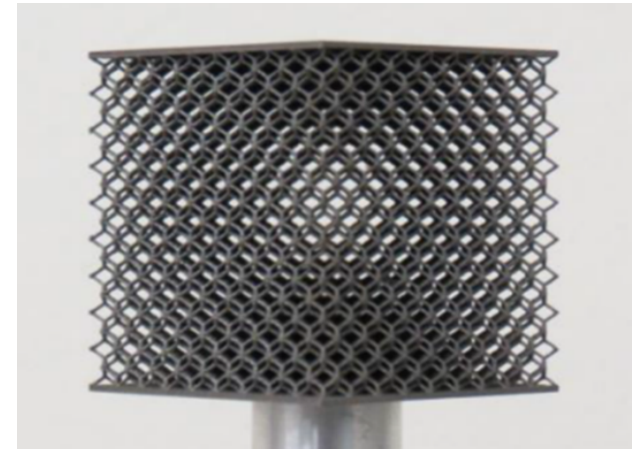
A complex lattice structure made of 316SS using an AM machine at LLNL.
