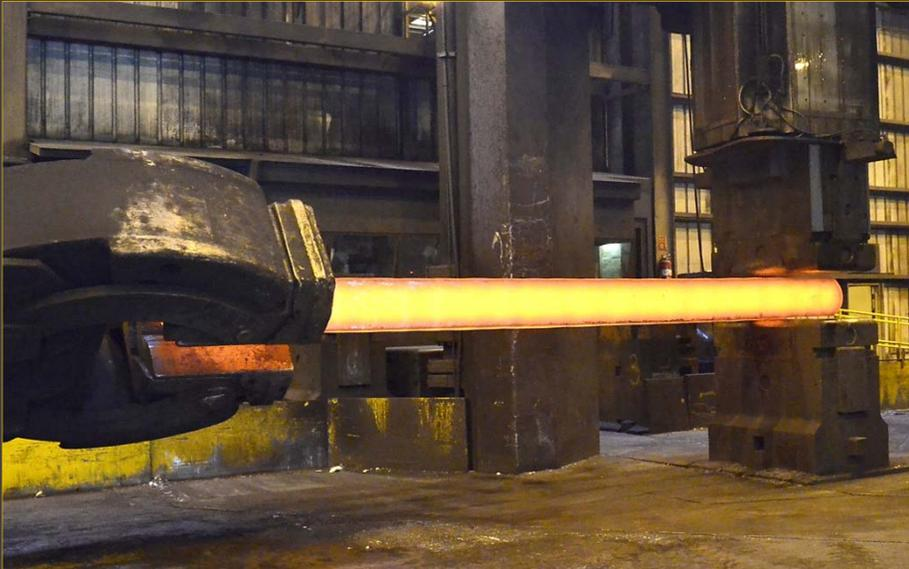
Forging of a tie-plate first article. The tie-plates are part of a substantial structural cage surrounding the central solenoid magnet.
