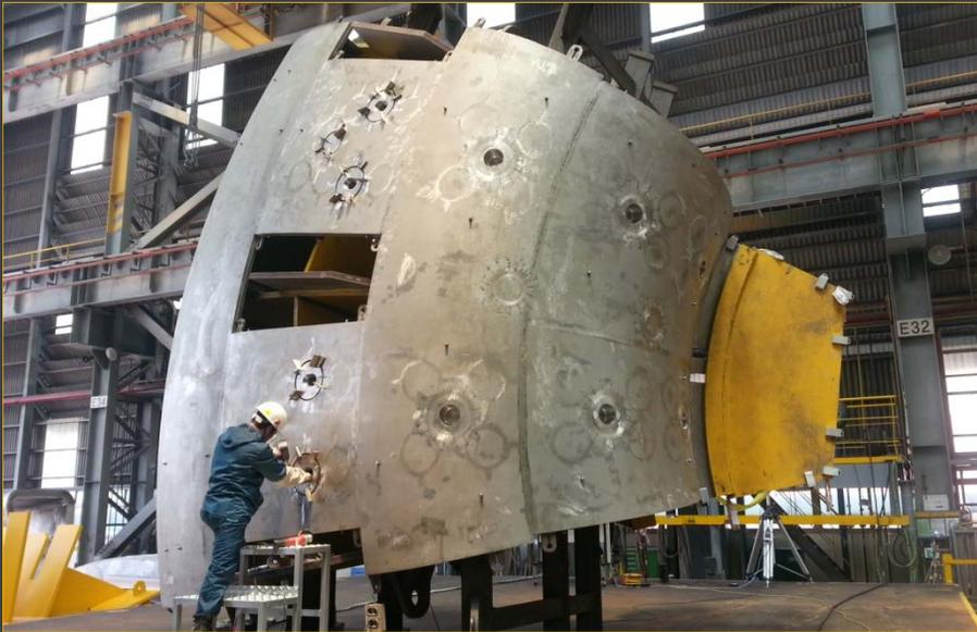
At Hyundai Heavy Industries, welding on the upper section of the inner shell for Sector #6.
