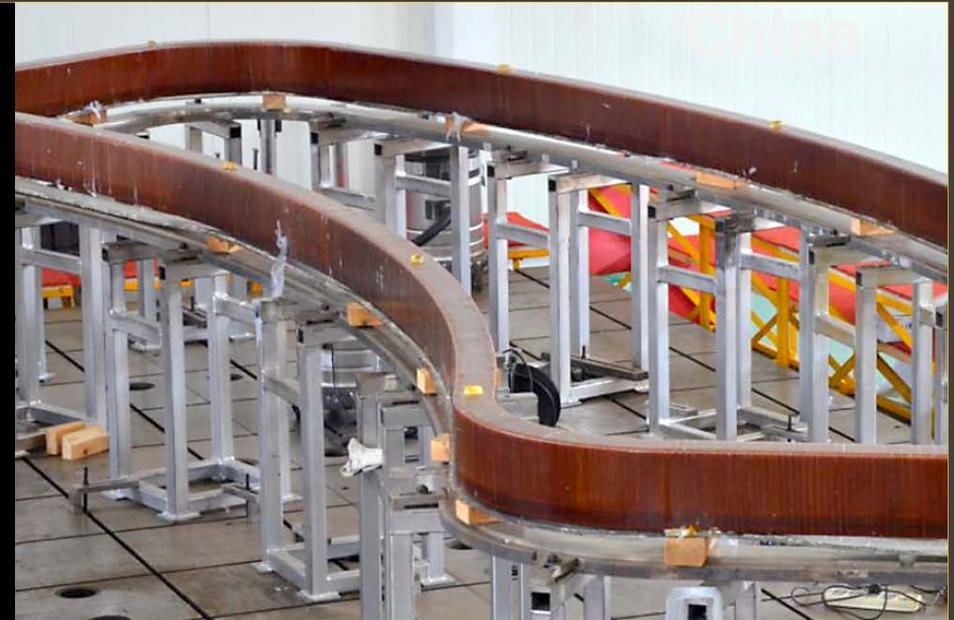
Correction coil vacuum pressure impregnation of a dummy double pancake at ASIPP.
