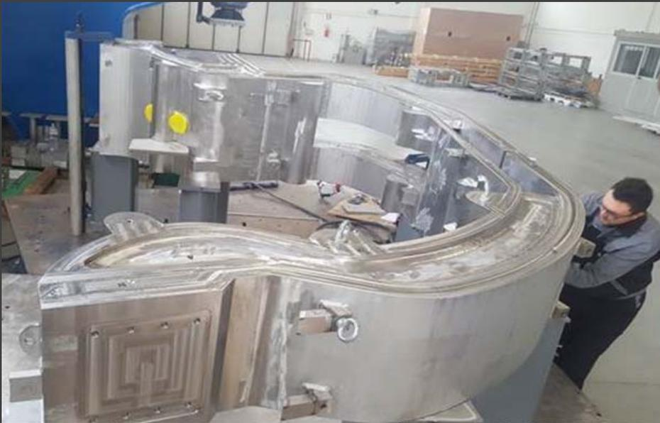
The manufacturing of the Full-scale Divertor Cassette Body Prototype is well advanced.
