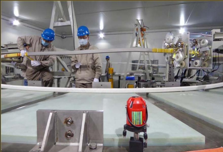
Tooling for Poloidal Field coil #6 (350 tons, 10 meters in diameter), is now complete and being commissioned.
