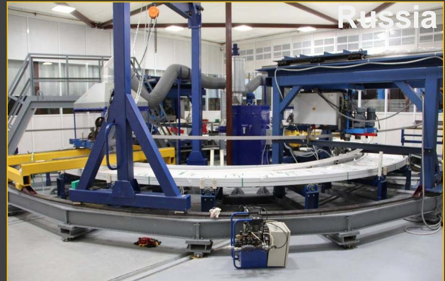
Winding of first double pancake for poloidal field coil #1 inside the clean room.
