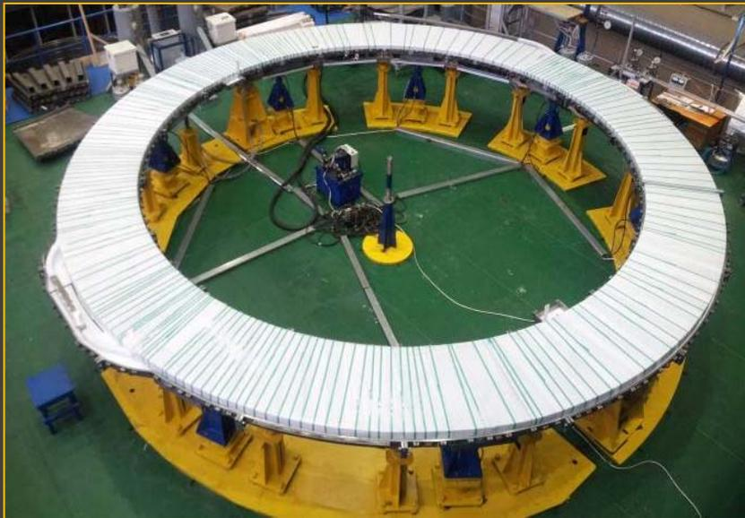
Fabrication and qualification tests of PF1 winding pack stack sample were successfully completed.
