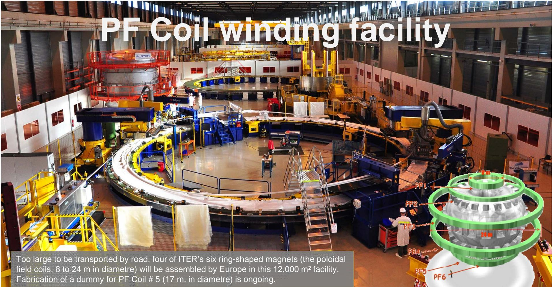
Too large to be transported by road, four of ITER's six ring-shaped magnets (the poloidal field coils, 8 to 24 m in diameter) will be assembled by Europe in this 12,000 m<sup>2</sup> facility. Fabrication of a dummy for PF Coil # 5 (17 m. in diameter) is ongoing.
