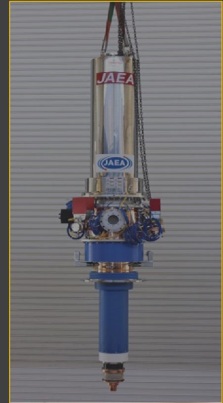
▲ Gyrotron prototype developed by RF-DA.
