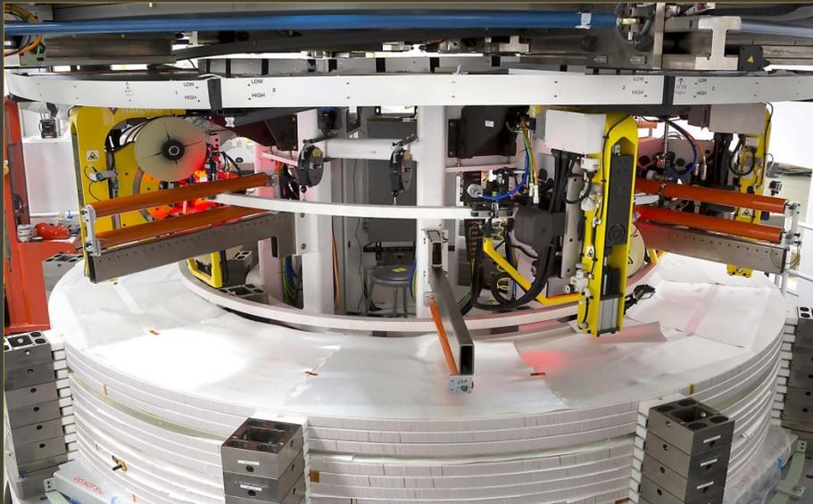
The turn insulation station wraps each bar of conductor with Kapton® fiberglass tape.
