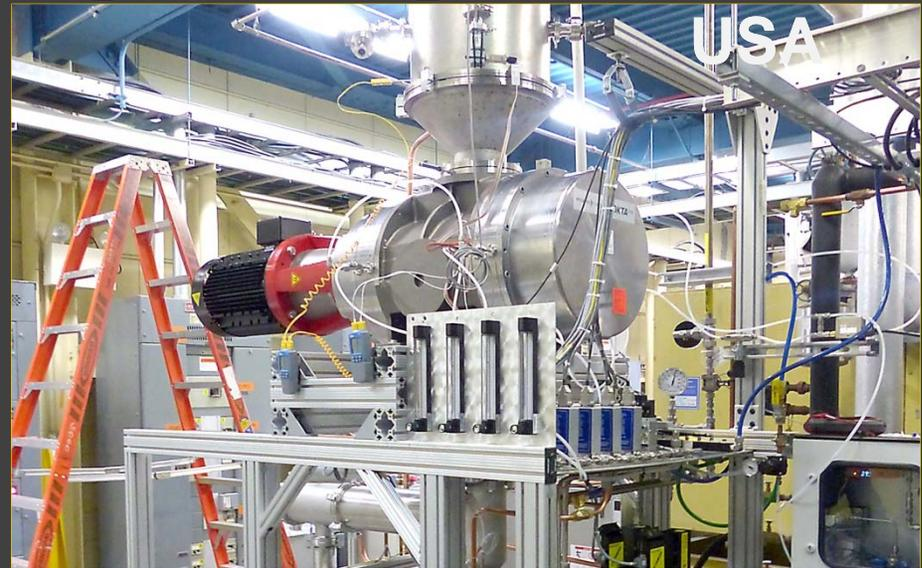
A roots pump prototype has been successfully tested at ORNL.
