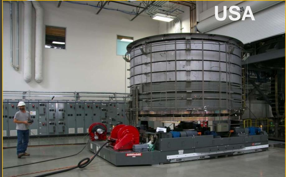
General Atomics is fabricating the 1000-ton Central Solenoid (CS). In April 2016, winding of the first CS module was completed.
