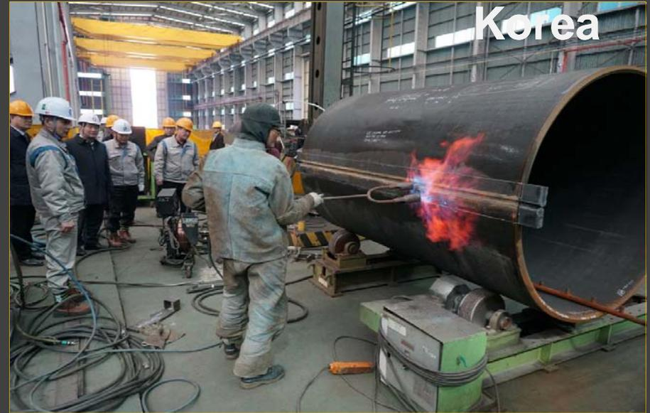
Welding operations of the first 800-ton Sector Sub-Assembly Tool, one of 128 purpose-built tools for assembly.
