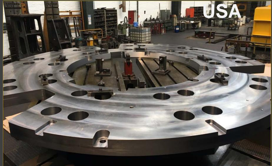
The top plate of the central solenoid assembly platform during fabrication at Robatel.
