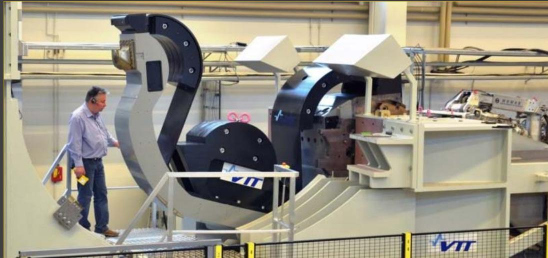
Due to the massive size of the ITER Tokamak components, as well as the intense neutron flux that will occur during operations, the ITER machine has required the development of cutting-edge robotics and remote handling tools, which will be used in both the assembly and operational phases.
