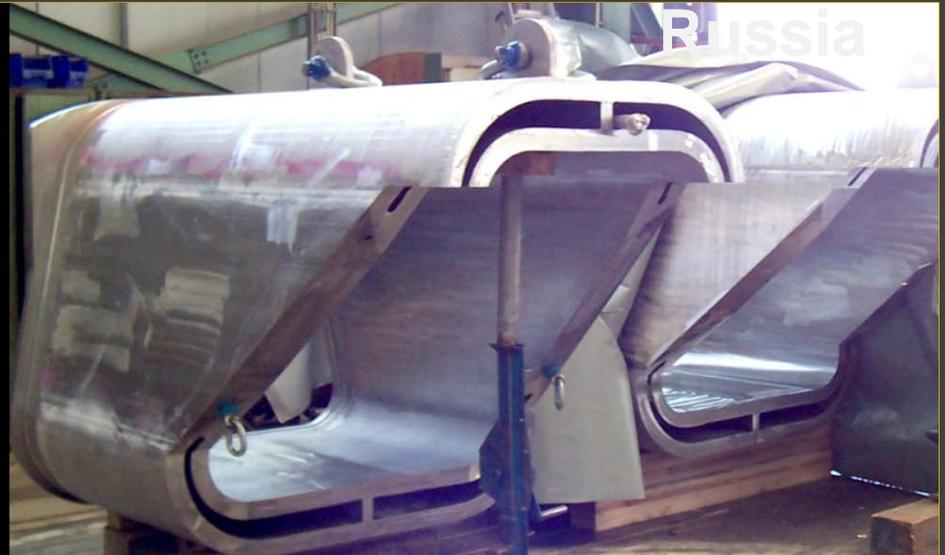
Russia completed its share of toroidal field conductor in June 2015, marking the end of a 5-year campaign to manufacture 28 production lengths (more than 120 tons of material).
