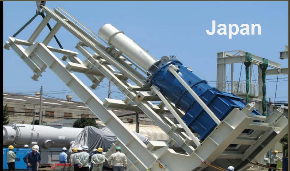
Series production of central solenoid conductor continues. 28 of 49 conductors have already been shipped to the US.
