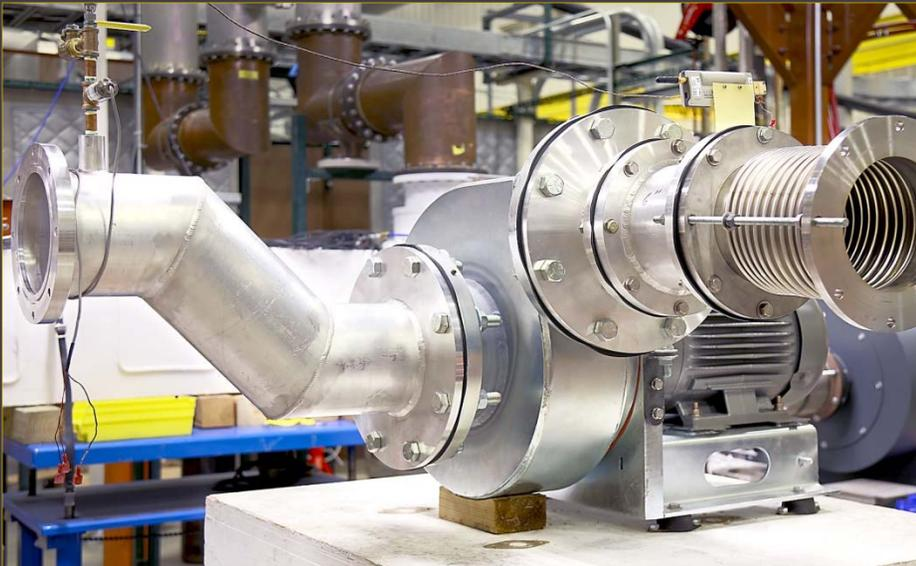
A blower for cooling transmission lines will be tested on the high-powered ORNL resonant test line.
