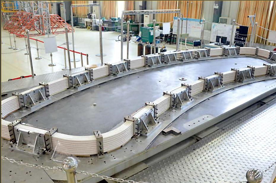
At ASIPP, the first-of-series, multiple-pancake bottom correction coil winding is prepped for the wrapping of ground insulation.
