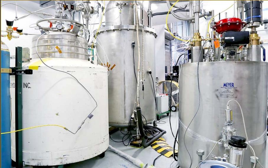
The cryoviscous compressor full-scale prototype was successfully tested at the ORNL Spallation Neutron Source cryo facility.
