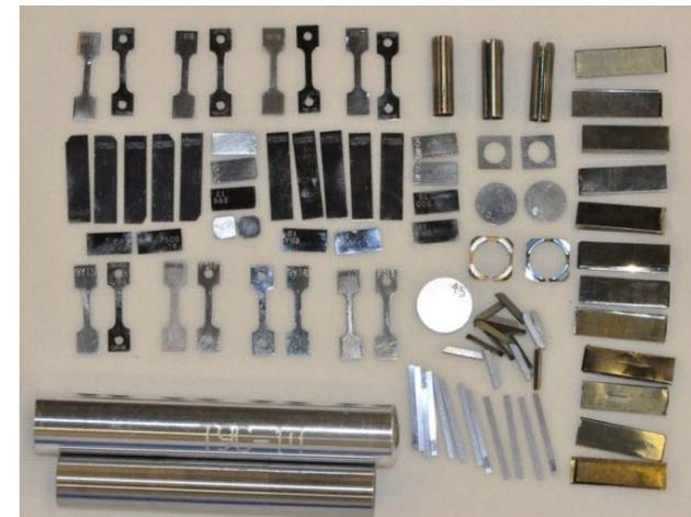
Several specimen types to be loaded into the irradiation capsules in lower left
