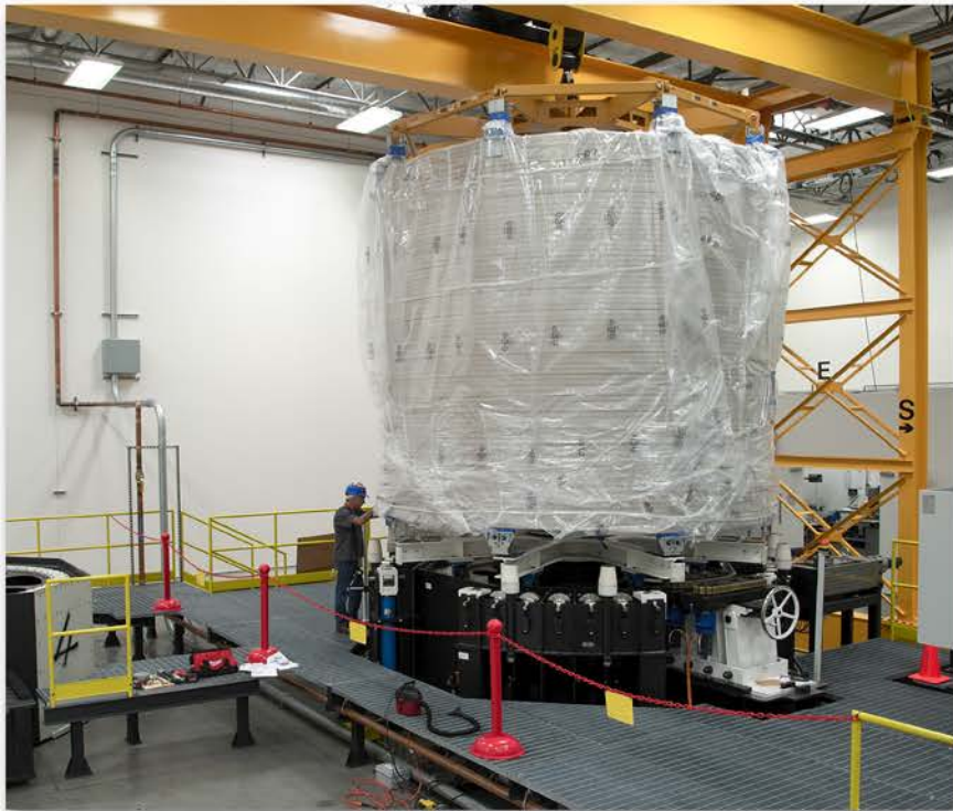
Dummy conductor shown loaded on winding machine – in prep for mock-up winding
