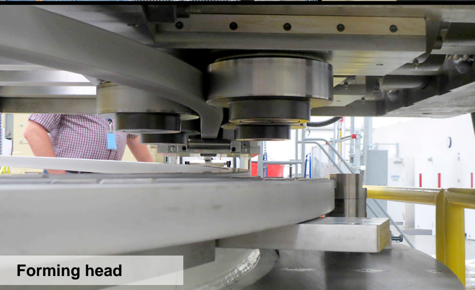
300m double pancake coil on winding table with cleaning, grit blast and de-spooler stations behind
