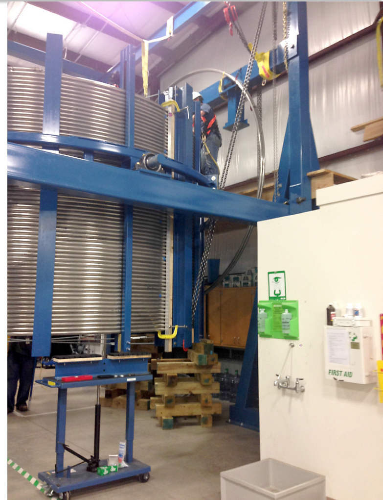
800 m Dummy Spool shown in turn-over frame at HPM
