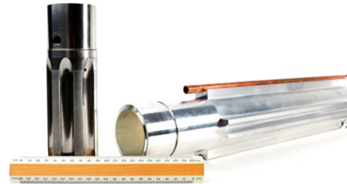
Aluminum waveguide and spiral corrugation tool
