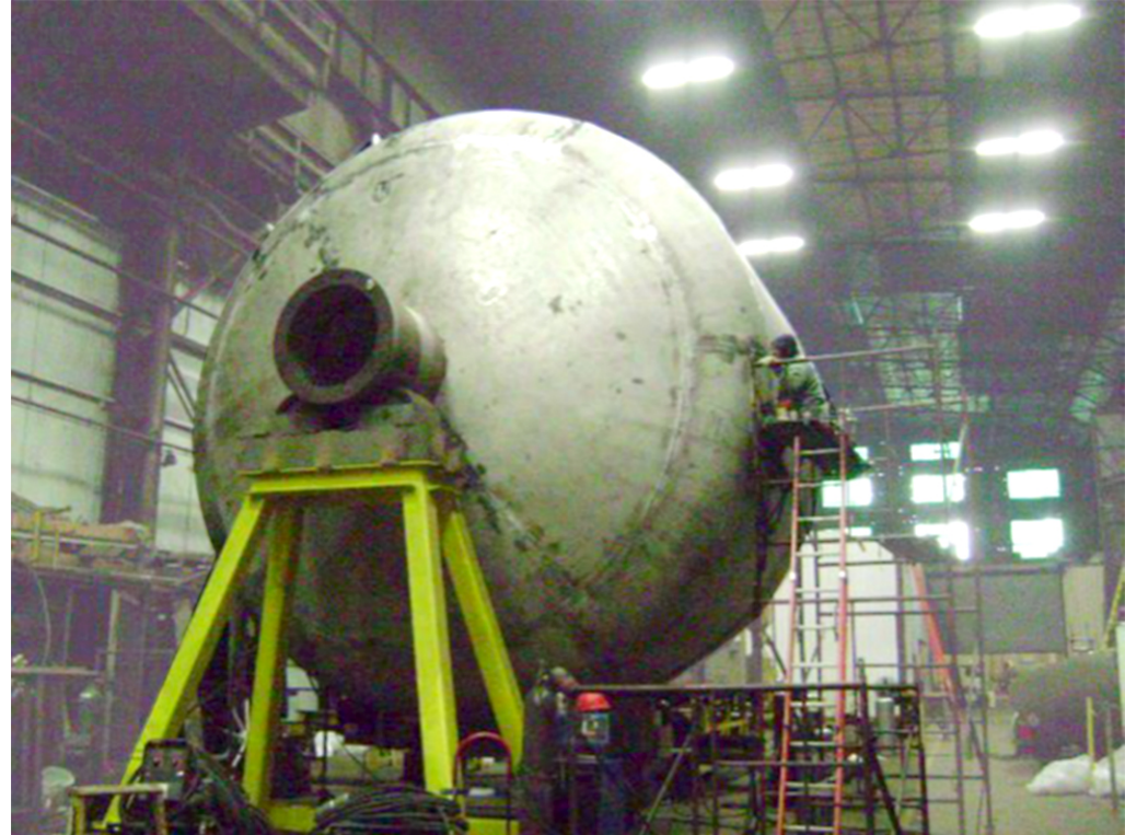
Drain tank heads and shells are being fitted and assembled at Joseph Oat Corporation (Camden, NJ). Photo: US ITER
