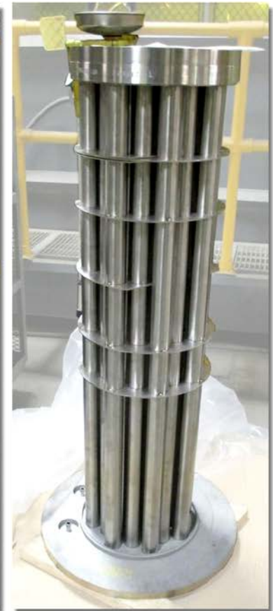
CVC pump inner tube bundle Photo: US ITER
