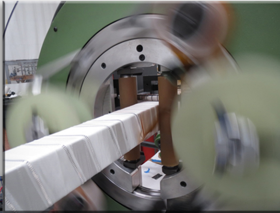
Automated machine wrapping of conductor bars at General Atomics (Poway, CA)
