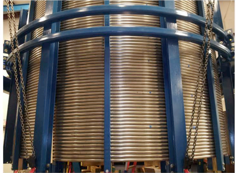
Completed 800 m dummy conductor at High Performance Magnetics (Tallahassee, FL)
