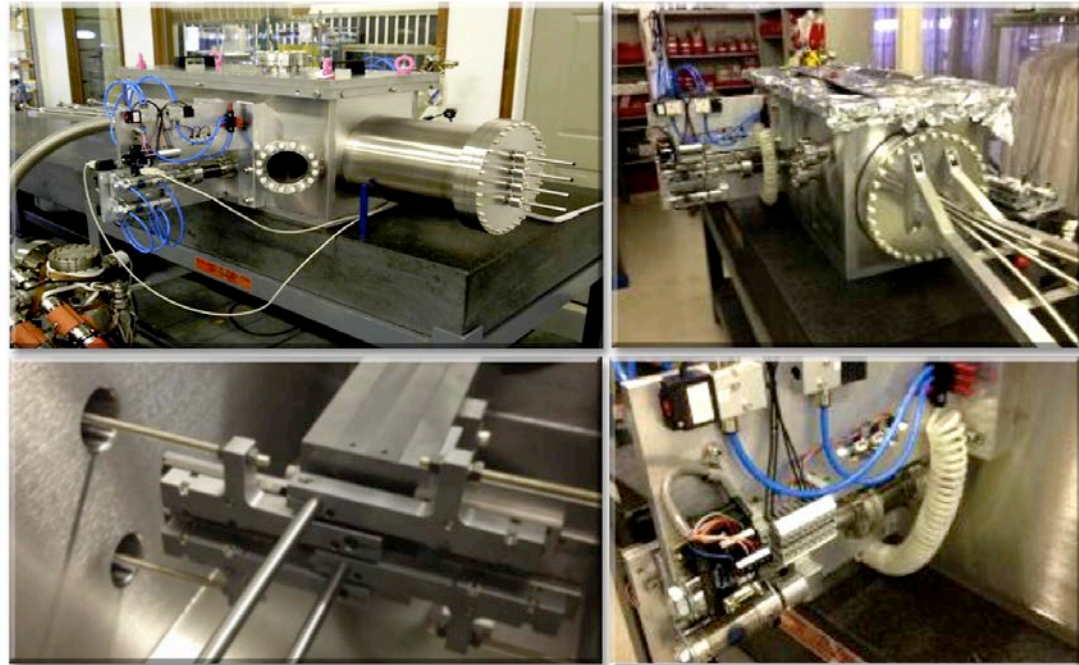
Pellet guide tube selector with internal views of actuators for routing pellets for multiple inputs to multiple outputs.
