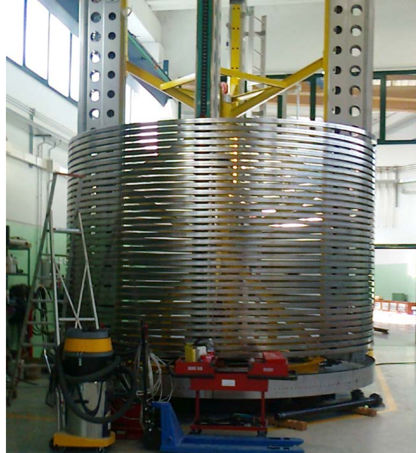
A copper dummy conductor fabricated for the PF1 coil
