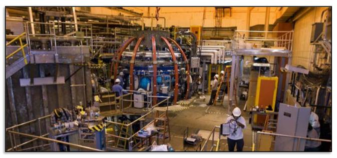
New solenoid, Inner TF bundle, TF joint, OH & Inner PF coils
