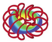
accompanying representation of a quasi-symmetric stellarator plasma enclosed by its magnet coils), several distinct types of quasi-symmetry have been identified theoretically, and one type has been experimentally tested with success at an exploratory level in a US device.
