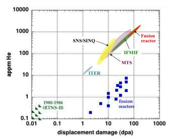
Comparison of 2-4 year helium and dpa production for ferritic steels in candidate irradiation facilities. Availabilities for SNS and MTS are actual, and projected for IFMIF.
