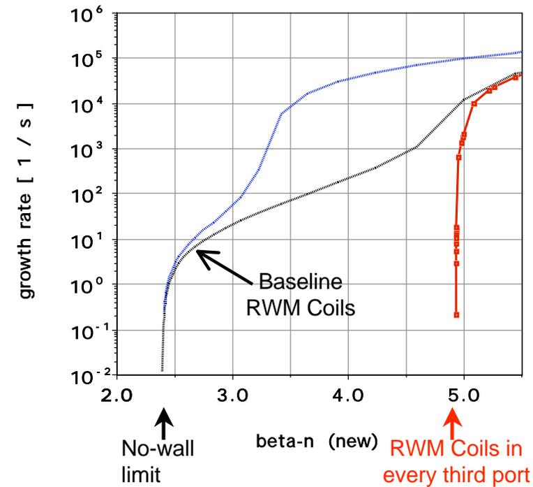
**FIRE-like RWM coils would have large stabilizing effect on  $n=1$**
