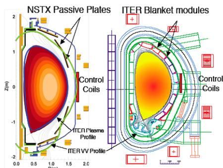
Fig. 2.2 Active mode control coils and passive plates for NSTX (left) and coils and (conducting) blanket modules proposed for ITER.
