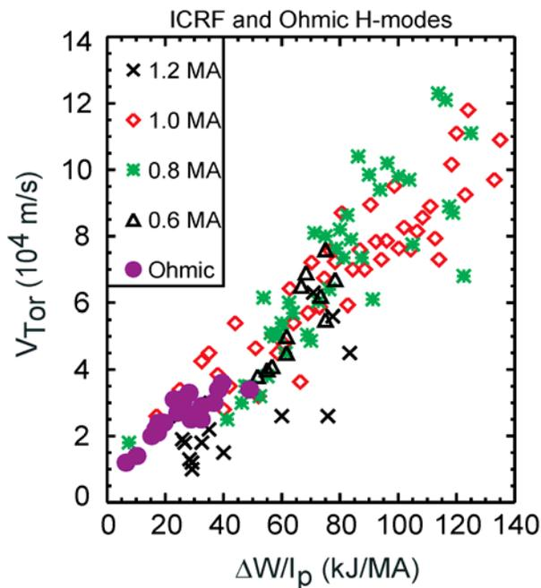
**Figure 8** Strong core rotation seen in high pressure C-Mod discharges. In most other tokamak experiments, transport-driven flows are masked by the presence of dominant externally applied torque from neutral beam injection.
