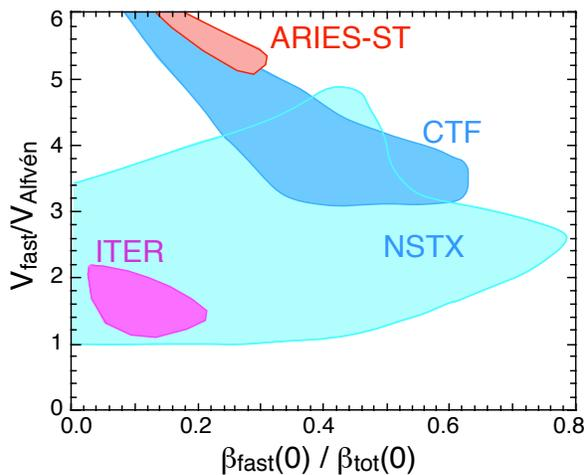
Fig. 4.1 Operating space for fast ions
