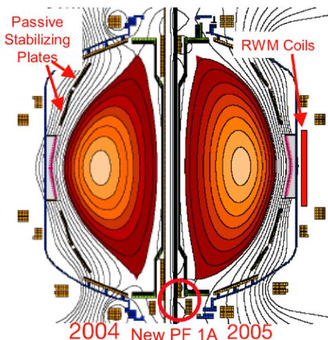
Fig. 7.2. New inner shaping coils and RWM Coils for the FY 05 operations
