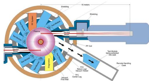
Fig. 6.2. Plan view of a CTF for rapid replacement of mid-plane test modules.
