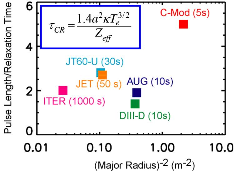
**Figure 2** Pulse length, normalized to current relaxation time ( $\tau_{CR}$ ) for high performance divertor tokamaks. For the operating devices,  $T_e = 6$  keV and  $Z_{eff} = 2$  are used to calculate  $\tau_{CR}$ . For ITER, 19 keV is assumed. Even inductively-driven shots in C-Mod routinely have pulse lengths greater than  $\tau_{CR}$ .
