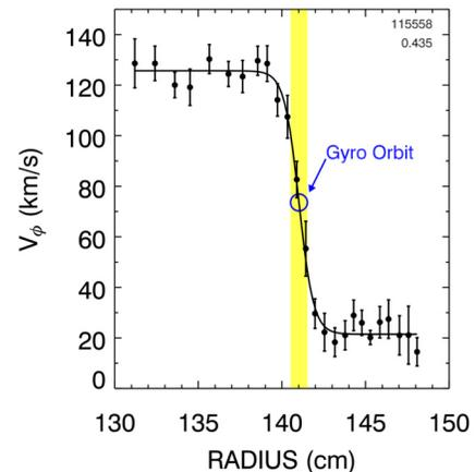
Fig. 3.1 Profile of  $V_\phi$  measured with *CHERS*, showing a shear layer with a scale length comparable to the ion gyro orbit size. The shear layer is formed between two magnetic islands.
