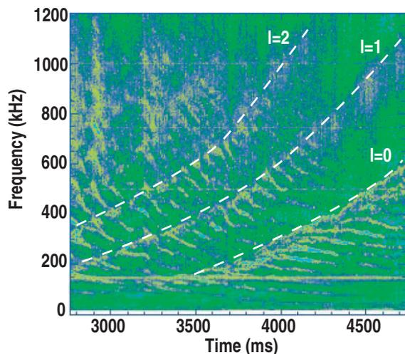
Fig. 8. FIR scattering shows a "sea of Alfvén eigenmodes" not visible on external magnetic diagnostics.
