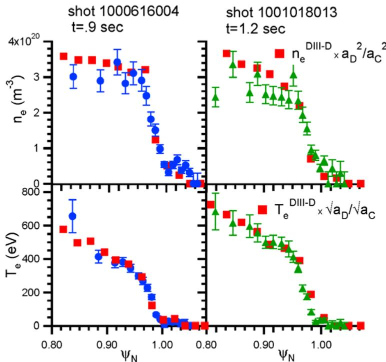
**Figure 7** Detailed dimensionless comparison of H-Mode pedestal structures on C-Mod and DIII-D show excellent agreement across the entire profile. The discharges are tuned so that they match at the top of the pedestal. The DIII-D data are scaled using the Kadomtsev constraints.
