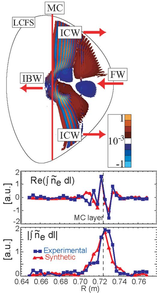
Figure 5 Comparison between TORIC simulations and experimental data measured with the Phase Contrast Interferometer (PCI) diagnostic. The top plot shows the contours of fluctuating electric field from the incoming fast wave, and the mode-converted (Bernstein and Ion-Cyclotron) waves in the core of the plasma. The code includes a synthetic simulation (red curve) of the PCI measurements (blue points).
