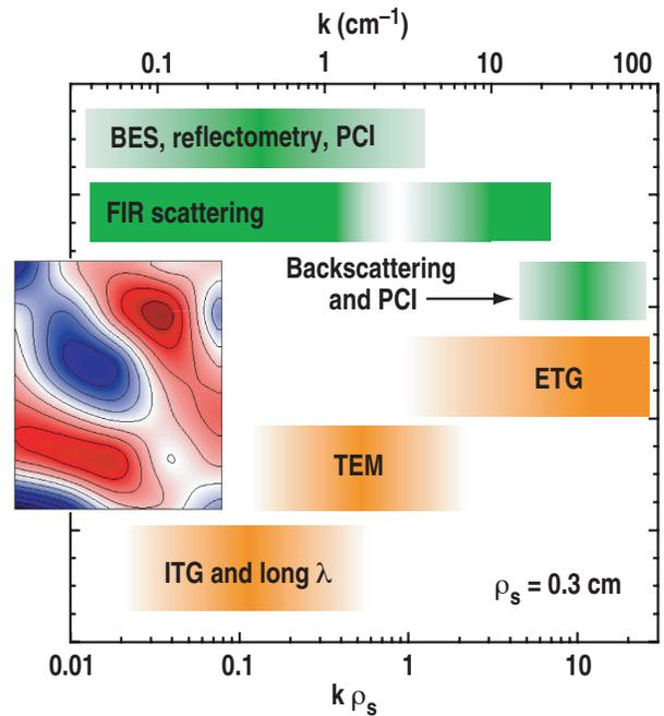
Fig. 4. DIII-D's comprehensive turbulence diagnostics cover all relevant spatial scales for transport physics. Turbulence cells from BES measurement.
