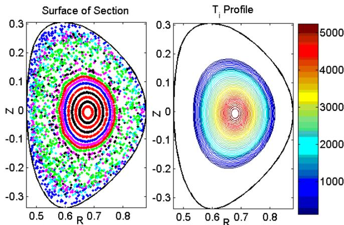
**Figure 4** NIMROD 3-D MHD simulation of gas-puff disruption dynamics in C-Mod. Edge cooling from the gas injection is imposed as an initial condition. Instabilities grow rapidly resulting in the inward propagation of B-field stochasticity which is faster than the gas velocity. The plot on the left shows flux surface breakup 11  $\mu$ s after the initial cooling. The plot on the right shows the dramatic cooling that results.
