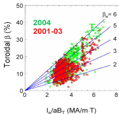
Fig. 2.1 Toroidal beta vs.  $I_p/aB_T$  from 2001 - 2004. High beta operation has become routine with the development of advanced shaping, control, and wall preparation. Also shown are lines of constant normalized beta.
