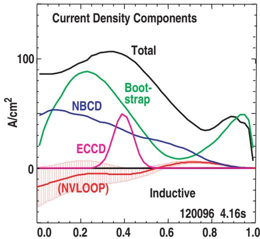
Fig. 3. 100% noninductive current achieved with good current profile alignment (loop voltage  $\approx 0$  everywhere).
