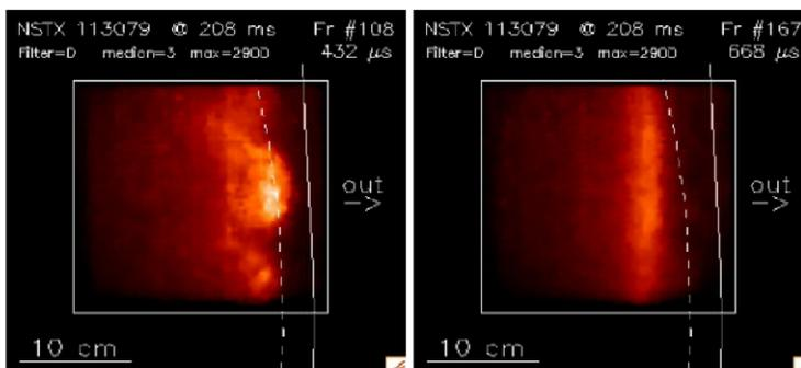
Fig. 5.1 Images of turbulent structures near the NSTX scrapeoff layer, before (left) and after an L-H transition
