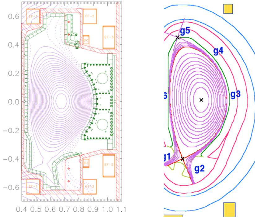
**Figure 1** C-Mod equilibrium (left) can match precisely the shape of the ITER design (right, shown scaled by 1/9 in linear dimension). The parameters for this actual C-Mod discharge were  $B_T = 5.3$  T,  $I_p = 1.6$  MA. The corresponding parameters for ITER are  $B_T = 5.3$  T,  $I_p = 15$  MA.
