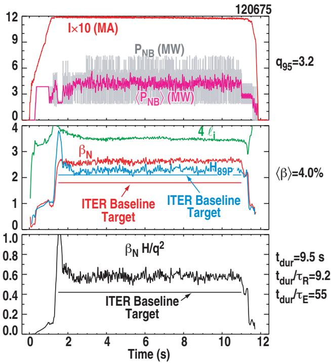
Fig. 1. Stationary high performance, at or above ITER baseline targets, in DIII-D advanced inductive scenario.
