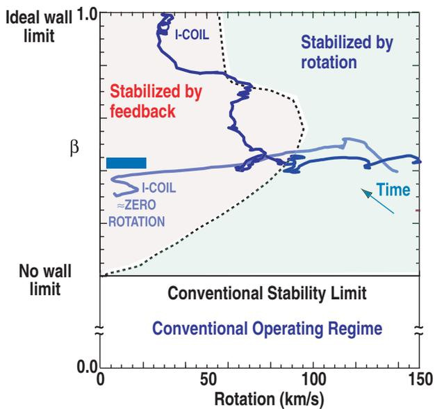
Fig. 5. RWM feedback control gives DIII-D unique access to the ITER-relevant regime of high beta and low rotation.
