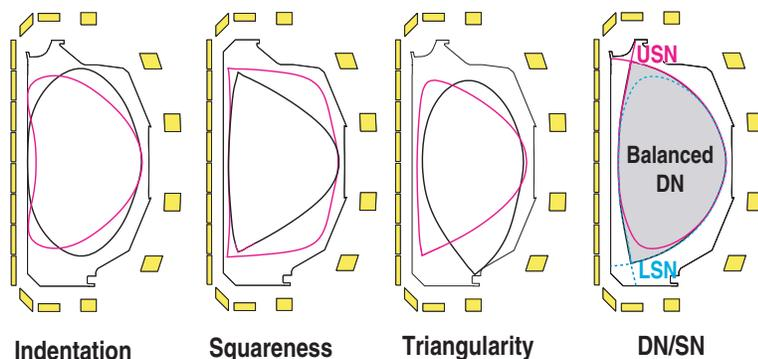
Fig. 9. DIII-D's unique shape control capability yields a wide spectrum of experimentally achieved discharge shapes.
