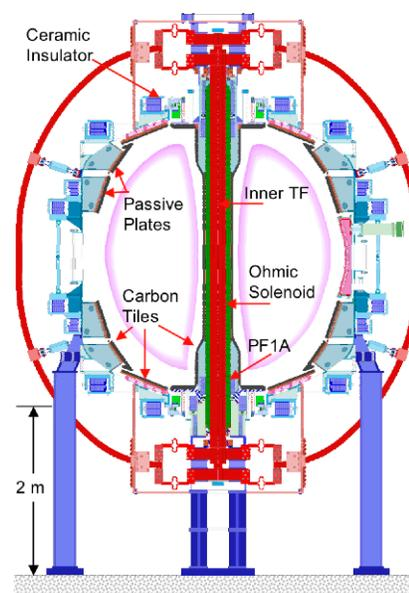
Fig.7.1 Cross section through NSTX
