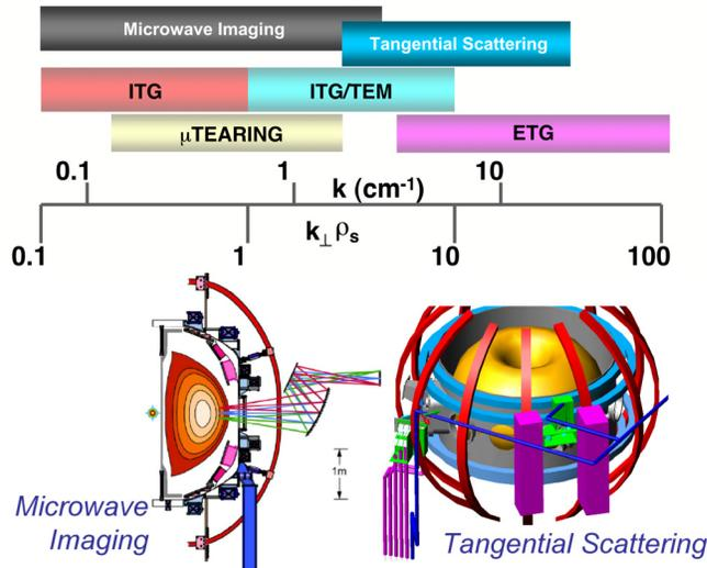
Fig. 3.2 The ranges of radial wavenumber that will be covered by the microwave imaging and tangential scattering diagnostics. Both systems (below) take advantage of the large port access and slender toroidal field coils in NSTX
