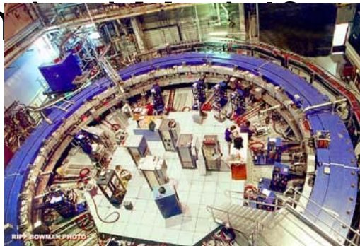
The muon storage ring at Brookhaven, home of the g-2 experiment's
