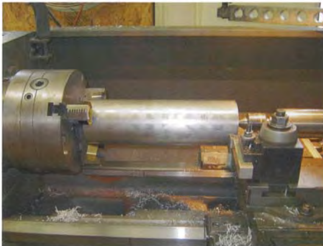
Figure 6: Cathode Tube (machining weld seat)
