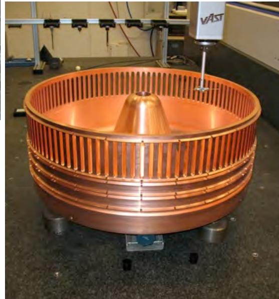
The “Coloseum” – RF surface and vacuum pumping apertures
