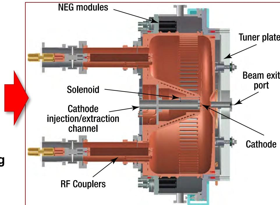
*The LBNL approach uses a CW photogun designed to meet all requirements*
