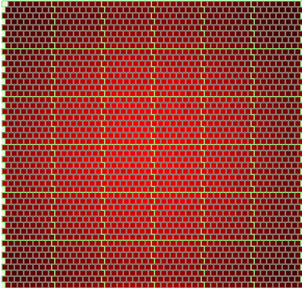
Response of entire  $48 \times 48$  pad detector and full acquisition system to uniform illumination with thermal neutrons. Neutron source is very close to detector window,  $d \sim 10\text{cm}$ , and thus there is a fall off of neutron intensity from center to the sides.
