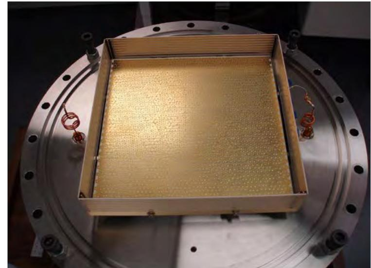
View of detector with window removed. Anode pad board and SANSROC are mounted on rear stainless steel flange, with drift field defining electrodes at edges
