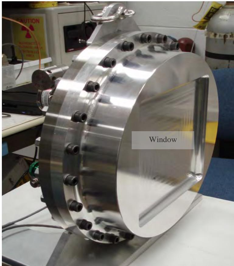
Completely assembled detector. Window defines sensitive area of 24 cm  $\times$  24 cm. Detector is sealed, with gas filling of  $^3\text{He}$  plus propane. Pump/puriifer maintains sufficient gas purity for long term operation.
