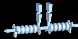
High current cavity showing the RF coupling and harmonic damping.
