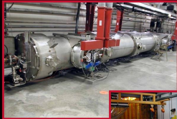
High Gradient Superconducting Linac installed at FEL for R&D tests.
