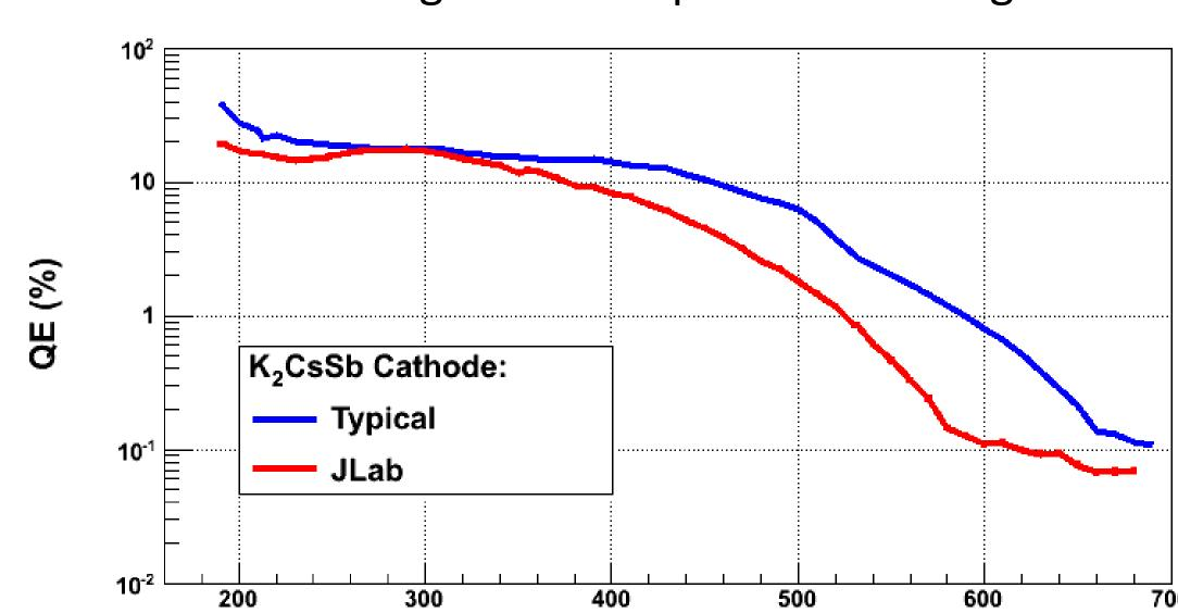
Wavelength (nm) During the Jlab cathode preparation, the K dispenser ran out, resulting in a top surface that has higher Cs concentration than stoichiometrically stable CsK<sub>2</sub>Sb.
