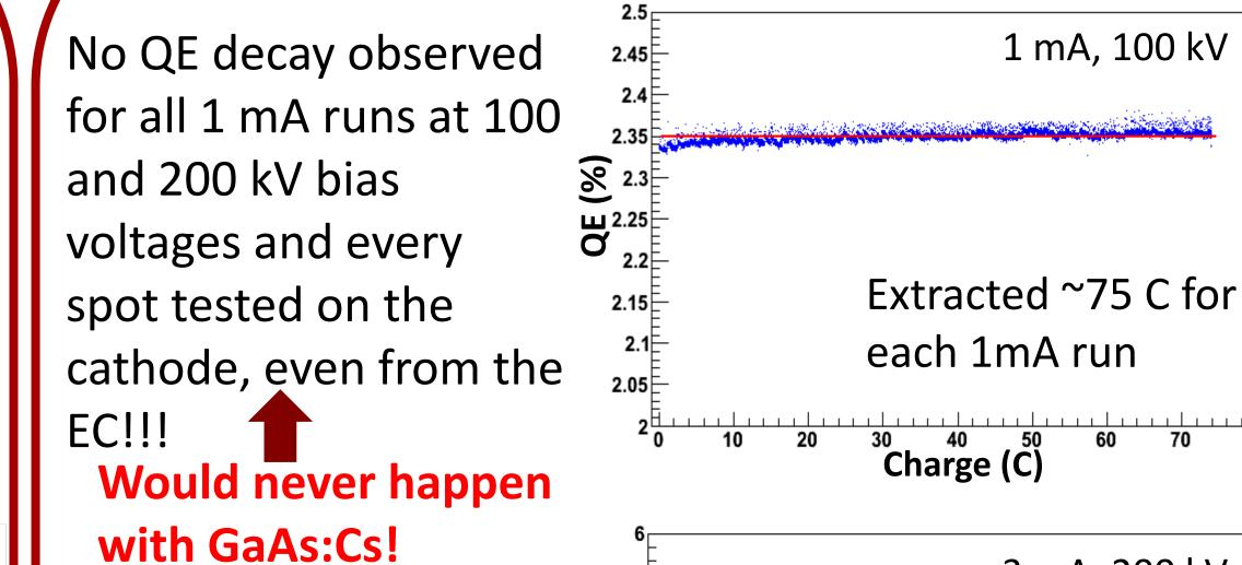
Cathode is very robust to short pressure increases in the beamline and gun. 825 C extracted before major vacuum event.
