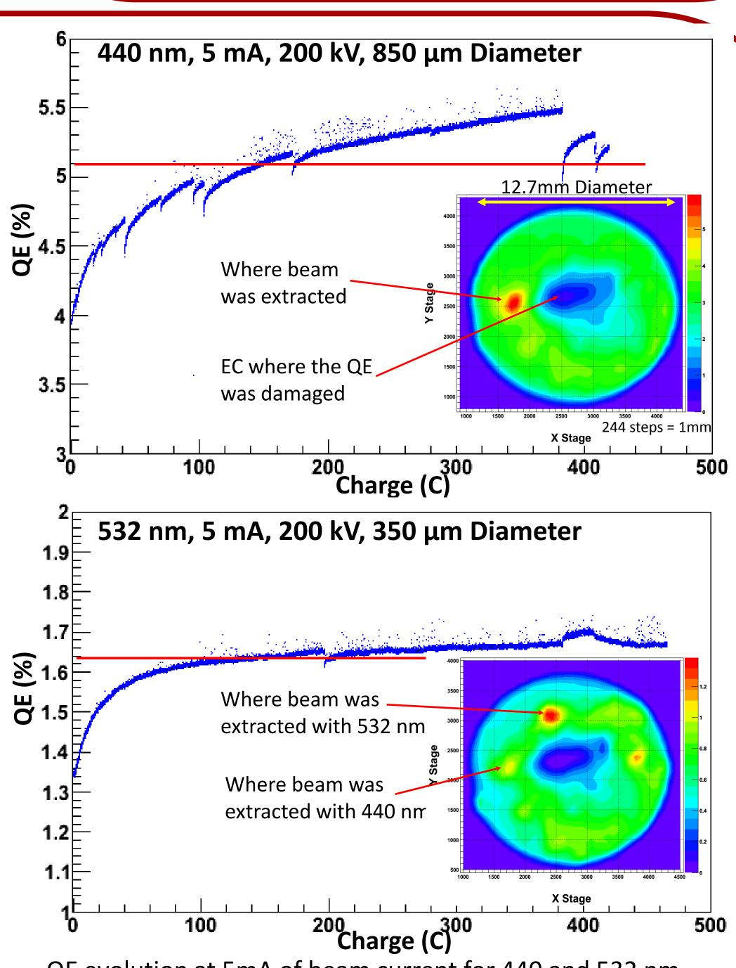
QE evolution at 5mA of beam current for 440 and 532 nm wavelengths. Inset shows a QE map of the photocathode after the ~24 run for each wavelength.
